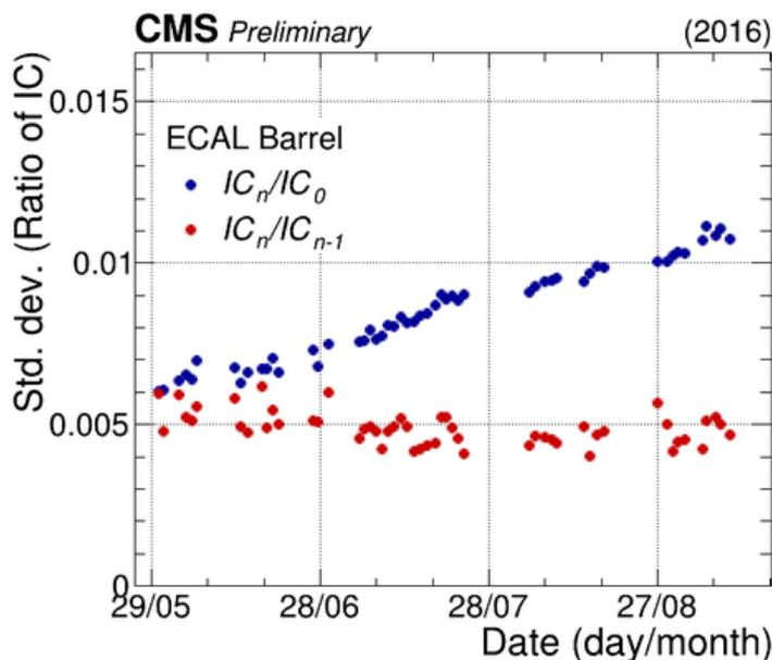
The plots show the relative variation of the intercalibration coefficients (IC) of the CMS ECAL during 2016 data taking. The IC are derived such that for channels located at the same pseudorapidity the average is one, while the intercalibration of different regions is then set
