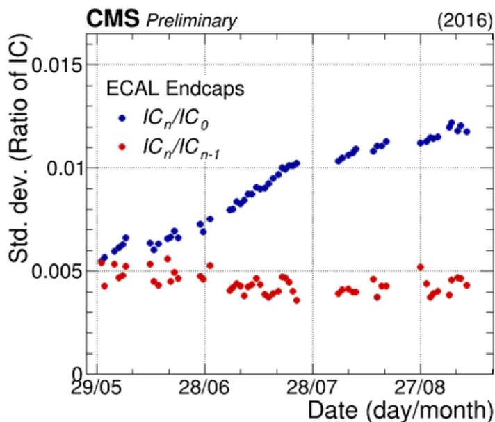
The plots show the relative variation of the intercalibration coefficients (IC) of the CMS ECAL
