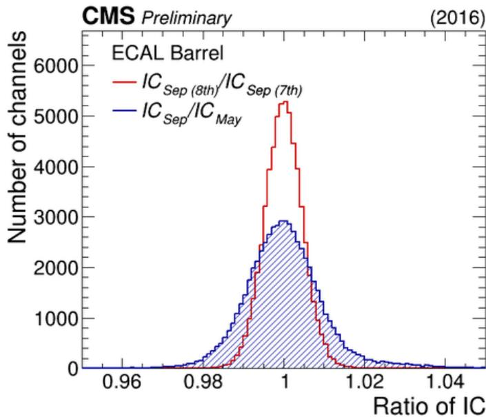
Distribution of the ratio of the intercalibration coefficients (IC) for all the channels in the CMS ECAL barrel ( $< 1.5$ ). The IC are derived exploiting the azimuthal symmetry of zero bias events: each IC set is derived with more than 80 million events collected over no more than two days which gives a statistical precision of about 0.4% on the IC ratio.
