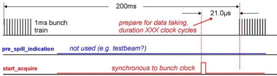
**Figure 3: Usage of control register bit 0 (CR0). With CR0='0', the command pre\_spill\_indication is not used. The DIF prepares for a measurement (e.g. turn on slab power) following the start\_acquire that is sent XXX clock cycles (to be defined) before the start of the bunch-train.**
