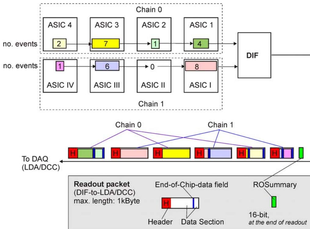
Figure 4: Output packets for a readout process for (exemplary) 2 readout chains.
