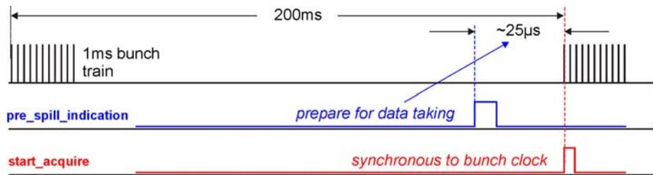
**Figure 2: Usage of control register bit 0 (CR0). With CR0='1', the command pre\_spill\_indication is used from the DIF to prepare for a measurement (e.g. turn on slab power). The start\_acquire is used for synchronous indication of the start of the bunch-train.**
