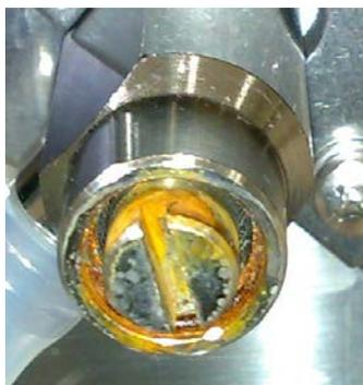
**Figure 3** The trace of corrosion on the drain valve after running the chiller with C6F14 and C6.
