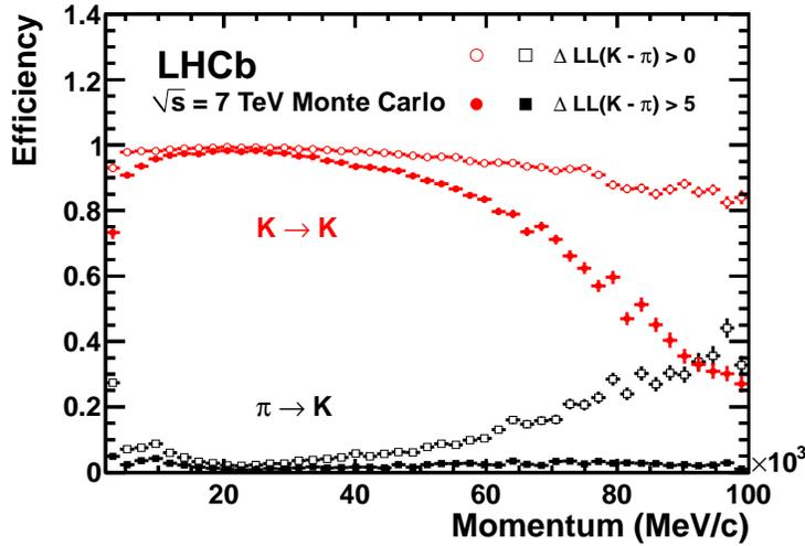
Figure 17: Kaon identification efficiency and pion misidentification rate measured using simulated events as a function of track momentum. Two different  $\Delta\log\mathcal{L}(K - \pi)$  requirements have been imposed on the samples, resulting in the open and filled marker distributions, respectively
