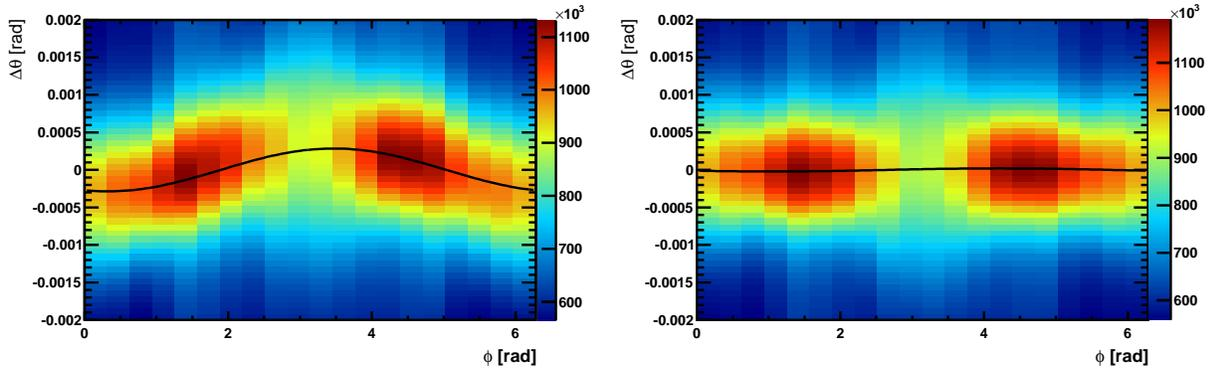
Figure 7:  $\Delta\theta_C$  plotted as a function of the azimuthal angle  $\phi$  and fitted with  $\theta_x \cos(\phi) + \theta_y \sin(\phi)$ , for one side of the RICH2 detector. The left-hand plot is prior to alignment, and shows a dependency of the angle  $\theta_C$  on the angle  $\phi$ . The right-hand plot is after the alignment correction, and  $\Delta\theta_C$  is uniform in  $\phi$
