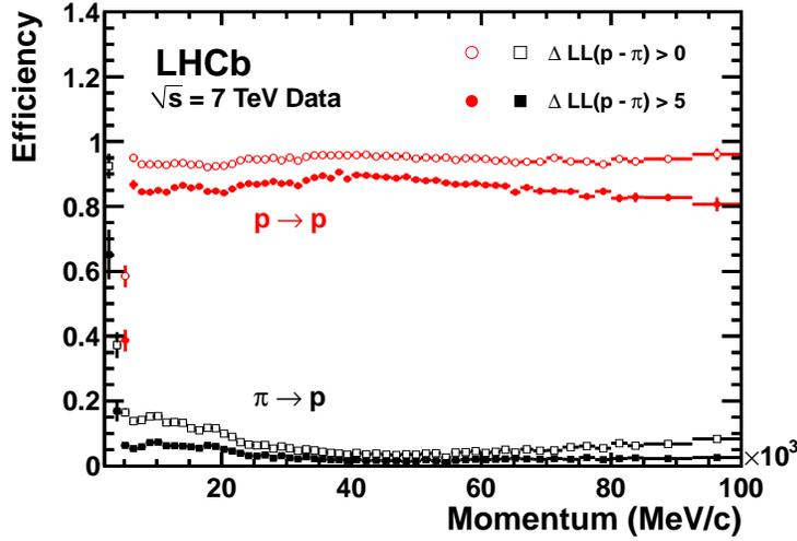
Figure 18: Proton identification efficiency and pion misidentification rate measured on data as a function of track momentum. Two different  $\Delta\log\mathcal{L}(p - \pi)$  requirements have been imposed on the samples, resulting in the open and filled marker distributions, respectively
