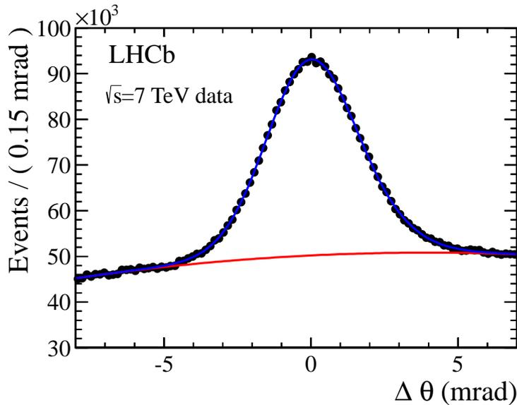
Figure 10: Distribution of  $\Delta\theta_C$  for  $C_4F_{10}$ . This plot is produced from kaons and pions from tagged  $D^0 \rightarrow K^- \pi^+$  decays in data selected with the criteria described in the text
