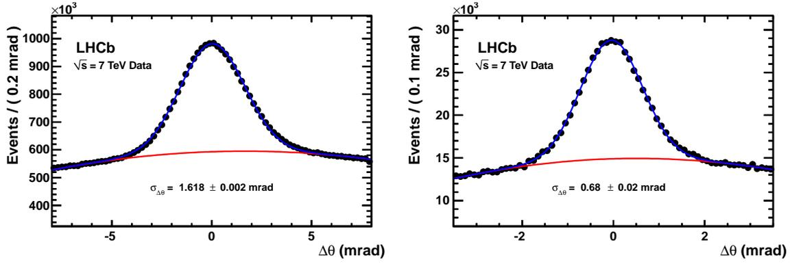
Figure 8: Single photoelectron resolution for the RICH1 (left) and RICH2 (right) gases, as measured in data for high momentum charged particles. The red line describes the background as determined from the fit using a polynomial function together with the Gaussian for the signal
