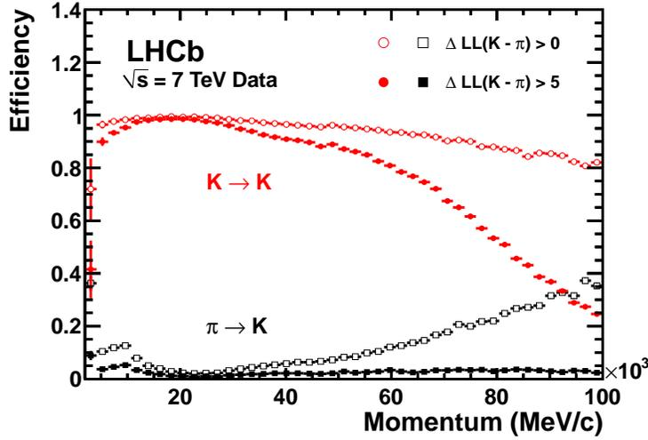
Figure 16: Kaon identification efficiency and pion misidentification rate measured on data as a function of track momentum. Two different  $\Delta\log\mathcal{L}(K - \pi)$  requirements have been imposed on the samples, resulting in the open and filled marker distributions, respectively
