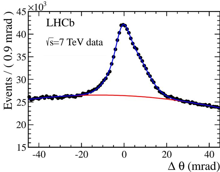
Figure 9: Single photoelectron resolution for the aerogel as measured in 2011 data with the  $pp \rightarrow pp\mu^+\mu^-$  events. The red line describes the background as determined from the fit using a polynomial function together with two Gaussians for the signal
