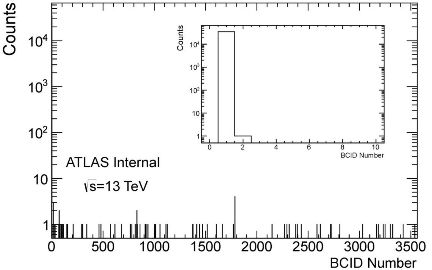
**Figure 1** – The measured number of OR-events by the LUCID fiber detector as a function of the bunch crossing number during one luminosity block in a fill with 13 TeV collisions recorded on the 21th of May 2015. The collisions were in the first bunch crossing and the inset plot shows that most of the counts are indeed recorded for the first BCID.
