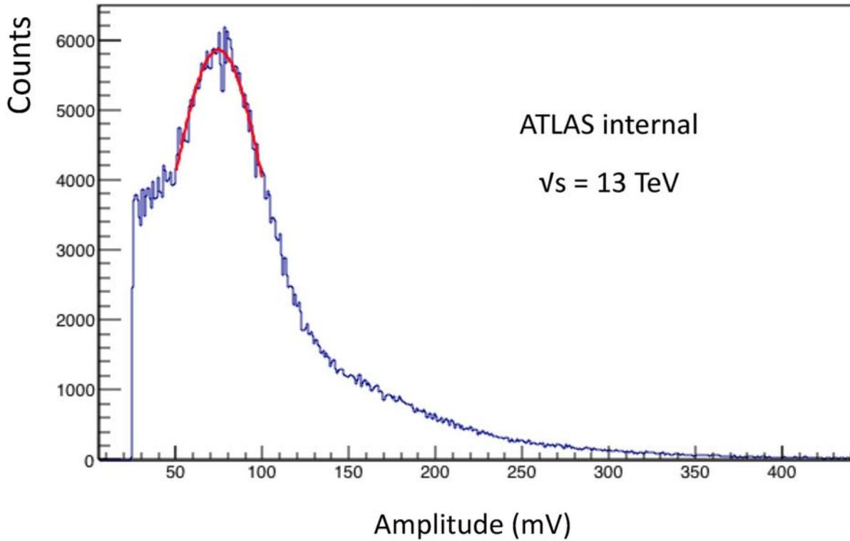
**Figure 4** – The pulseheight distribution from one photomultiplier in the LUCID detector during a 13 TeV run recorded on the 21th of May 2015. The Cerenkov light created in the quartz window of the photomultiplier produces a clear peak in the amplitude distribution that has been fitted by a Gaussian distribution (in red). Only signals above a threshold defining a particle hit are plotted in the figure.
