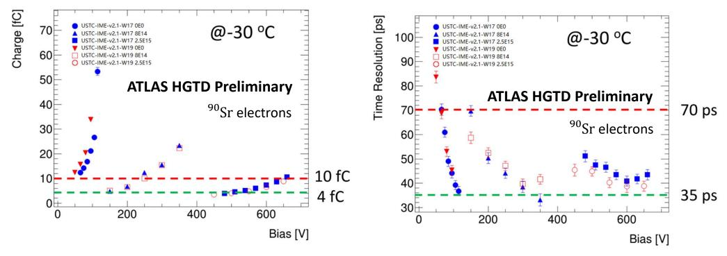
Collected charge (left) and time resolution (right) of USTC-IME-v2.1 at fluences of 0, 8E14, 2.5E15  $\rm n_{eq}/cm^2$ . This  $\beta$ -scope test is performed at USTC. The target collected charge is 4 fC and time resolution of 50 ps.
