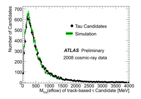
The invariant mass of the charged and neutral decay products where the energy deposits associated to tracks have been replaced by the track momenta as measured in the Inner Detector.
