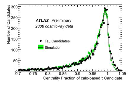
The ratio of the transverse energy of calo-based tau-jet candidates within a cone of  $\Delta R < 0.1$  to their transverse energy within a larger cone of  $\Delta R < 0.4$
