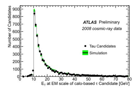
Transverse energy of calo-based tau-jet candidates at the electromagnetic scale (no hadronic calibration applied). The  $E_T$  at the EM scale is a safe variable used for identification in first data.
