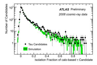
The fraction of the uncalibrated transverse energy deposited in the electromagnetic calorimeter in a cone  $0.1 < \Delta R < 0.2$  around the direction of the tau candidate with respect to the total energy in the cone of  $\Delta R < 0.4$ .
