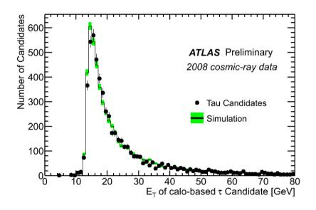
Transverse energy of calo-based tau-jet candidates. Seed topojets must have  $E_T > 10 \text{ GeV}$  and  $|\eta| < 2.5$ . Cell energies in the hadronic calorimeter are calibrated to the hadronic scale.
