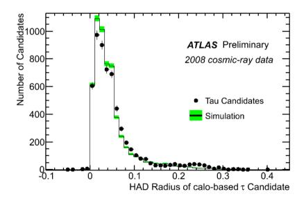
The radius of energy deposits in hadronic calorimeters for calobased tau-jet candidates. This variable corresponds to the lateral development of hadronic showers.
