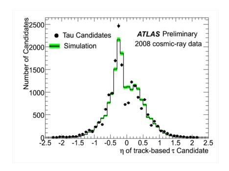
Pseudorapidity of track-based tau candidates. The double-peak structure is connected to the two construction shafts. The general distribution and basic features of the data agree with the simulation; smaller characteristics, however, are not reproduced as well. This plot identifies areas for improvement in the simulation.
