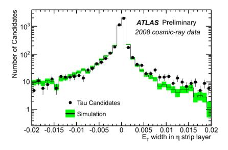
The transverse energy weighted width of tau candidates in the  $\eta$  direction in the first layer of the electromagnetic calorimeter.
