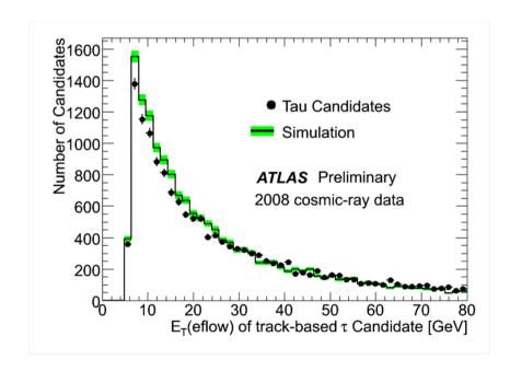
Transverse energy of track-based tau-jet candidates. The energy is determined using an energy flow algorithm. In this method the energy deposit in cells is divided into two categories, as coming from the neutral and charged components of a tau-jet. After calculation of the component energies, the energy coming from the track is replaced by the transverse momentum of that track from the Inner Detector.
