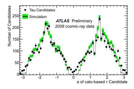
The phi direction of calo-based tau-jet candidates. The majority of events are from seed jets that have a large energy deposit in a single cell; this cell defines the direction of the tau candidate.
