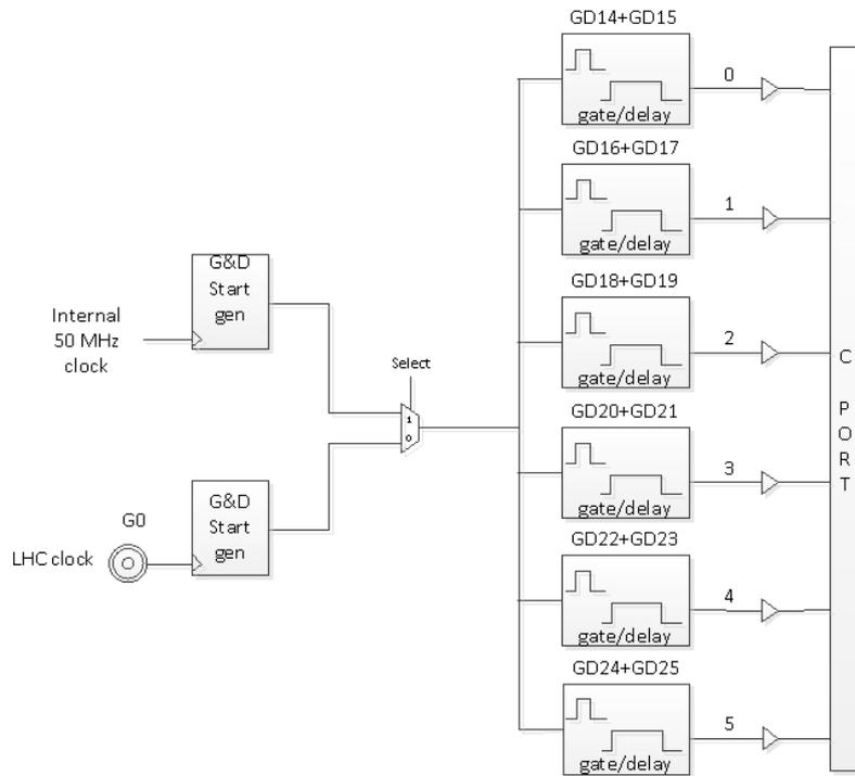
Figure 5: Test generators (drive of C port)
