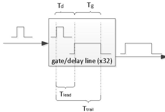
Figure 1: Internal Gate and Delay parameters
