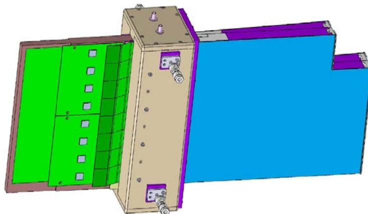
Figure 1: View of a single BGV detector module. The SiPMs sit in an enclosure box providing thermal insulation (brown). The two connections for the cooling pipe are visible. The connections visible on the top are for circulation of dry air to avoid frost/condensation inside the box on the cold elements.
