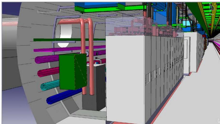
Figure 4: Proposed location of the cooling unit in UA43. The cooling unit is shown in grey and the transfer line in pink.
