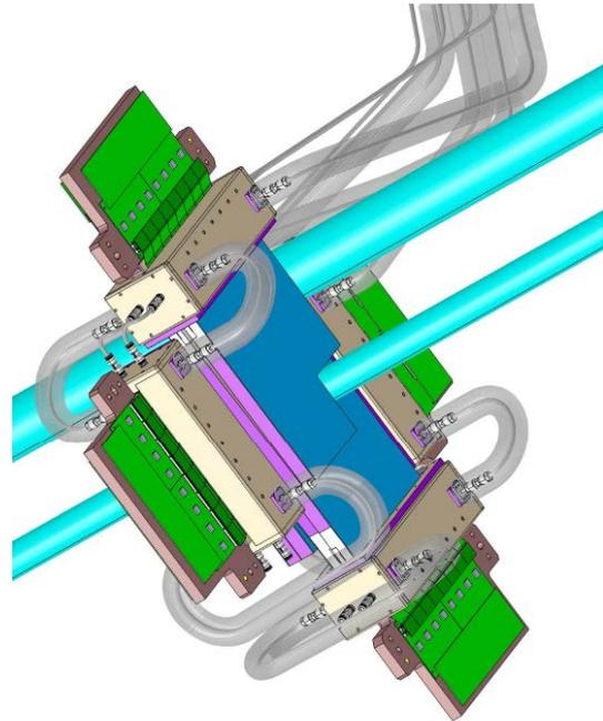
Figure 7: Left: manifold for the distribution of the cooling liquid to the BGV modules. Right: view of detector modules around the beam pipe (in cyan) with the cooling tube connections (in grey).
