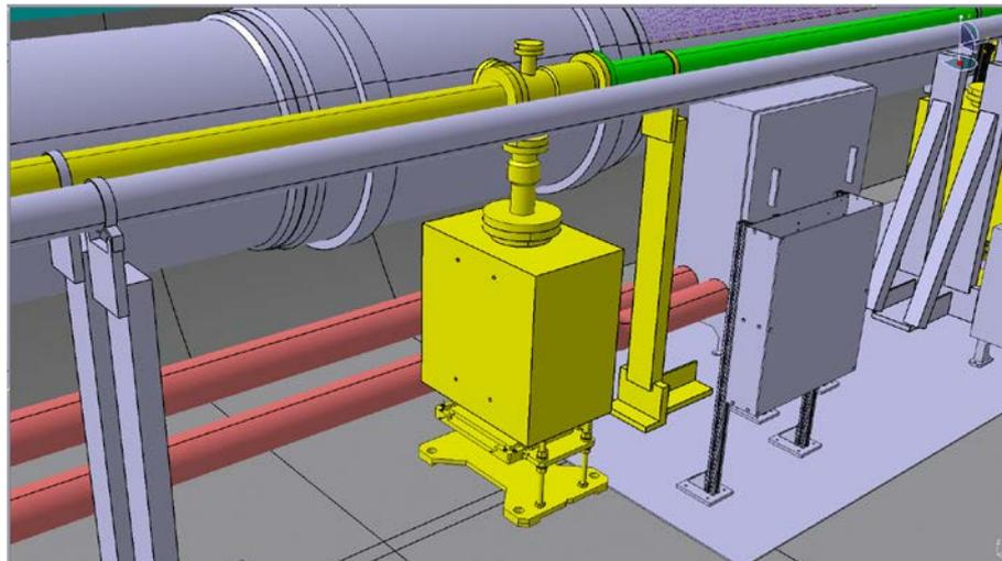
Figure 6: Connection of the cooling transfer line to the cooling distribution manifold near the BGV setup in RA43 (Preliminary).
