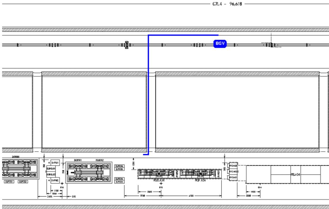
Figure 3: Proposed location of the chiller unit and path of the transfer line between UA43 and RA43.
