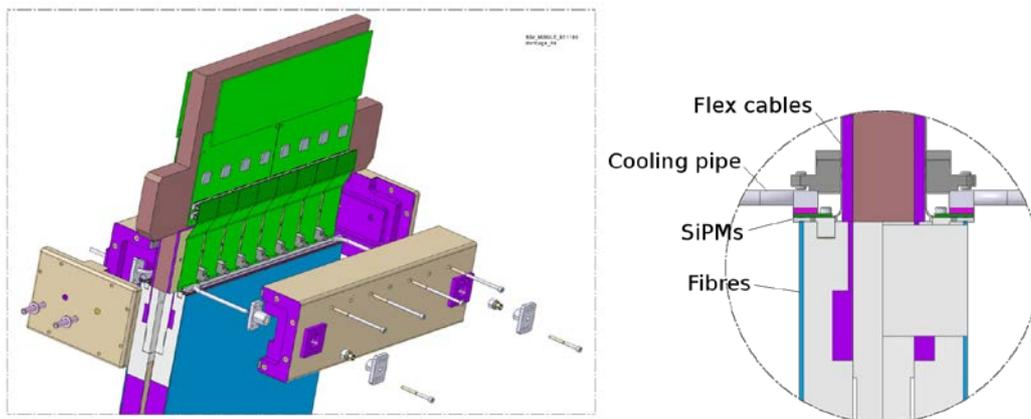
Figure 2: Exploded (left) and transverse (right) views of the BGV detector module. The cooling pipe is glued to an aluminium plate and pressed against a row of 8 SiPM by a system of springs.
