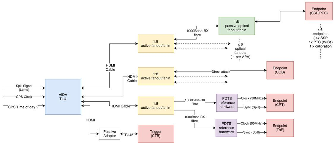
Figure 1: Block Diagram of protoDUNE-SP timing system
