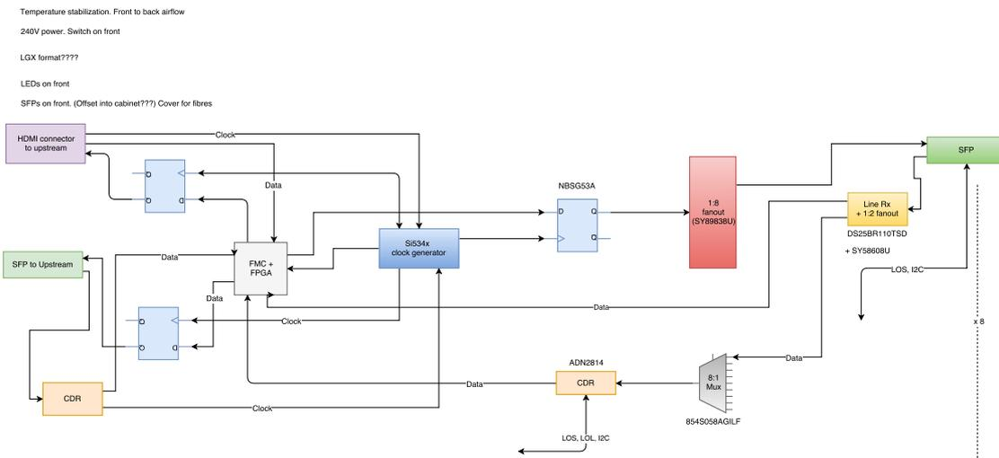
Figure 2: Block Diagram of PDTS Active Fanout
