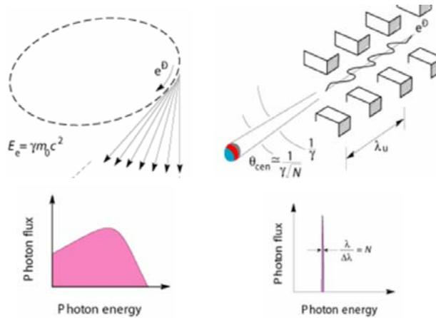
Figure 11: The two methods of x-ray production using accelerator technology. On the left the “Synchrotron radiation” technique and on the right “FEL”, free electron laser method.
