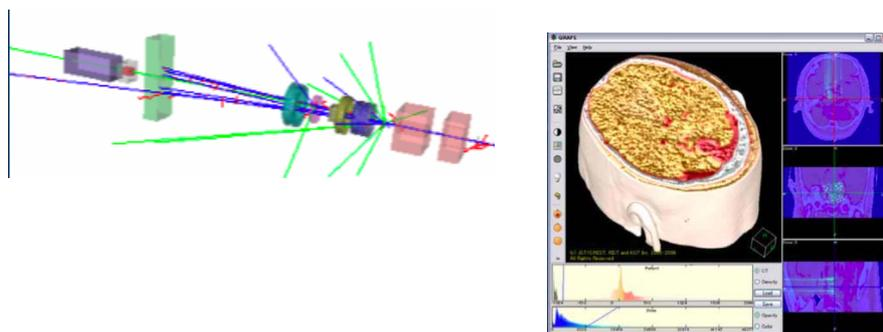
Figure 7: The software which was developed initially for tracking particles through the detectors (left) was adapted for medical physics applications such as visualization of PET data (right).
