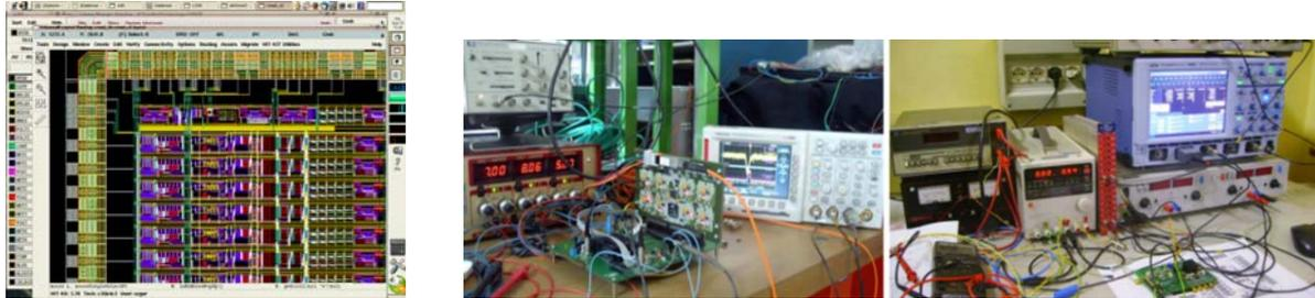
Figure 6: Left: Design of a Radiation Hard application specific integrated circuit (ASIC) Right: The setup to test for the manufactured ASIC.
