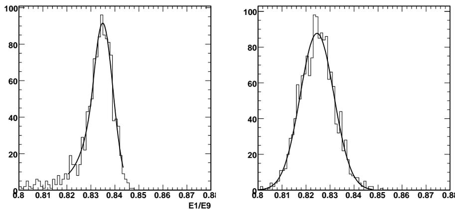
**Figure 8.** Distribution of the simulated E1/E9 ratio from the test beam data from 120 GeV electron (left) and with FastSim with the default setting of the Molière radius (right).
