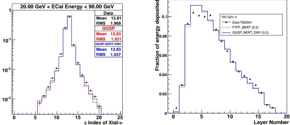
**Figure 3.** (left) Transverse shower profile of  $100 \text{ GeV}/c \pi^-$  and (right) longitudinal shower profile of  $150 \text{ GeV}/c \pi^-$  compared with the predictions of GEANT4 using different physics lists.
