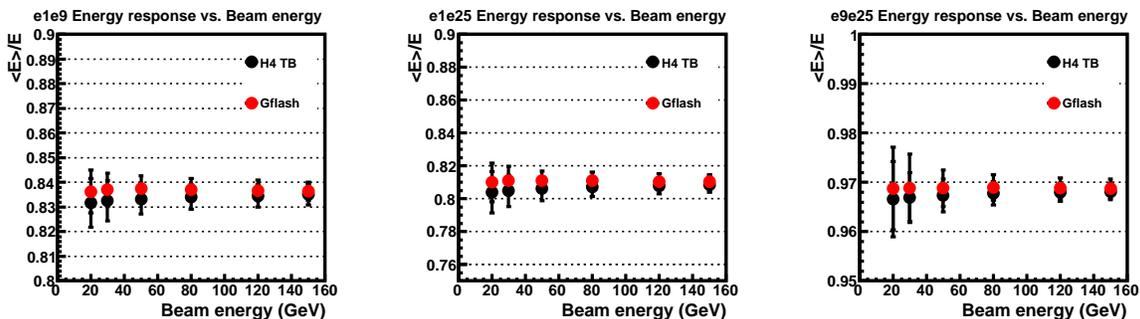
**Figure 5.** Mean fractional energy deposit in  $1 \times 1$  (E1),  $3 \times 3$  (E9) and  $5 \times 5$  (E25) crystal matrices in the test beam data and tuned GFLASH parameterization.
