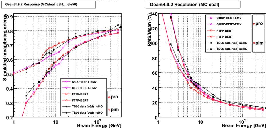
**Figure 2.** (Left) Mean energy responses of  $\pi^-$  (shown as circles) and protons (shown by squares) are compared with the predictions of QGSP\_BERT\_EMV physics list (shown by empty points) as a function of beam momentum. (Right) Energy resolutions for  $\pi^-$  and proton are compared with predictions of Full Simulation as a function of beam momentum.
