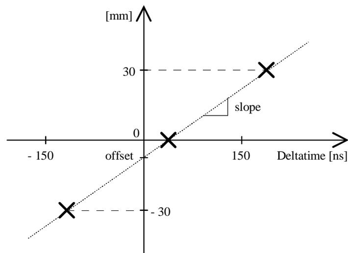
Figure 4. Calibration principle.
