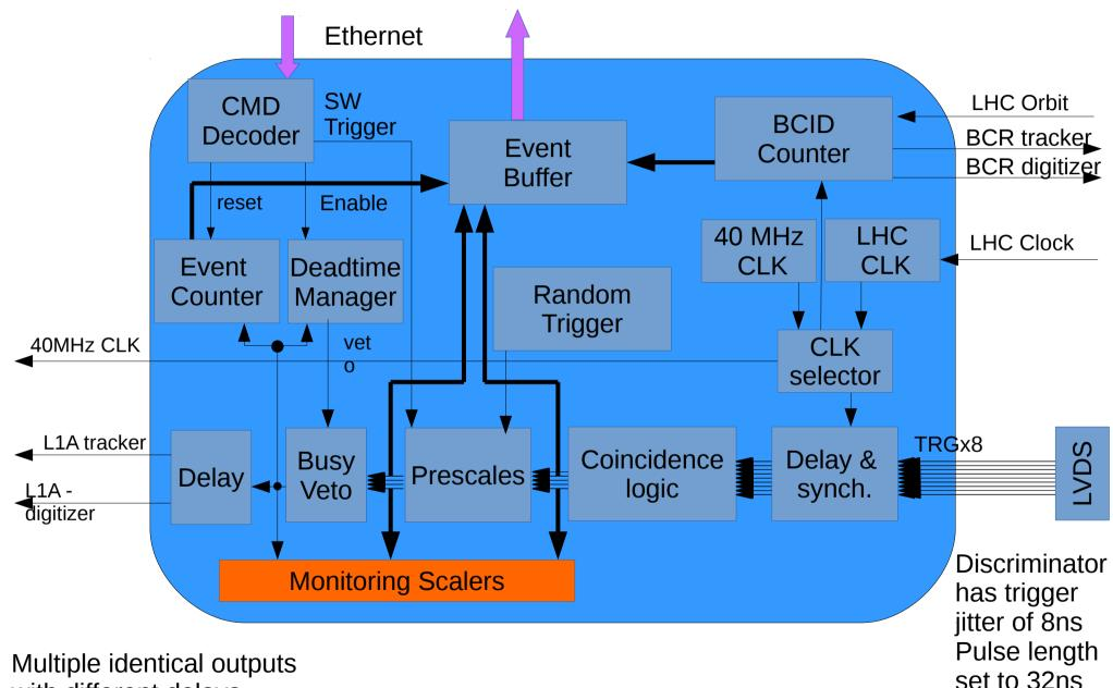
Multiple identical outputs with different delays for tracker and digitizer
