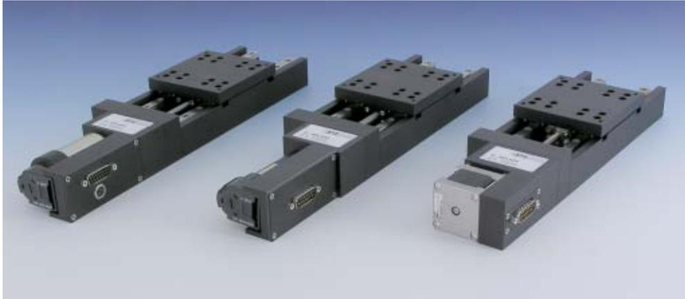
Figure 1: Different motor versions of the M-403 linear stage family with 100 mm travel range (from left): M-403.4PD (DC-motor/Active Drive(TM)), M-403.4DG (DC-motor/gearhead) and M-403.42S (stepper motor)
