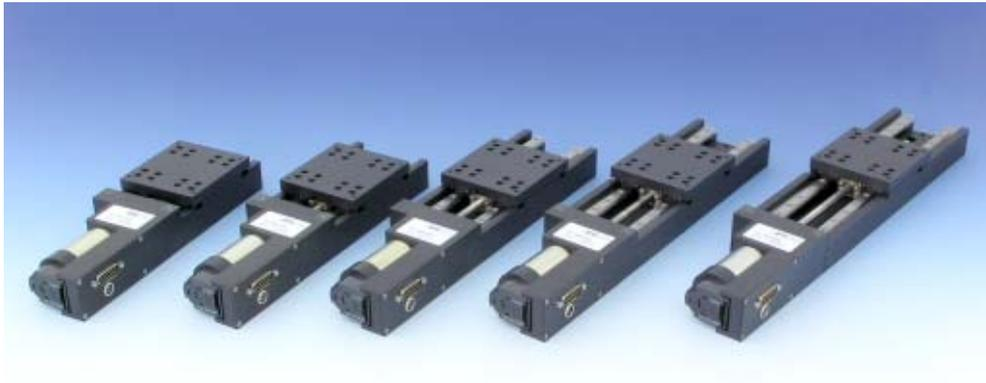
Figure 2: M-403 linear stage versions (from left): M-403.1PD, M-403.2PD, M-403.4PD, M-403.6PD and M-403.8PD provide travel ranges from 25 to 200 mm
