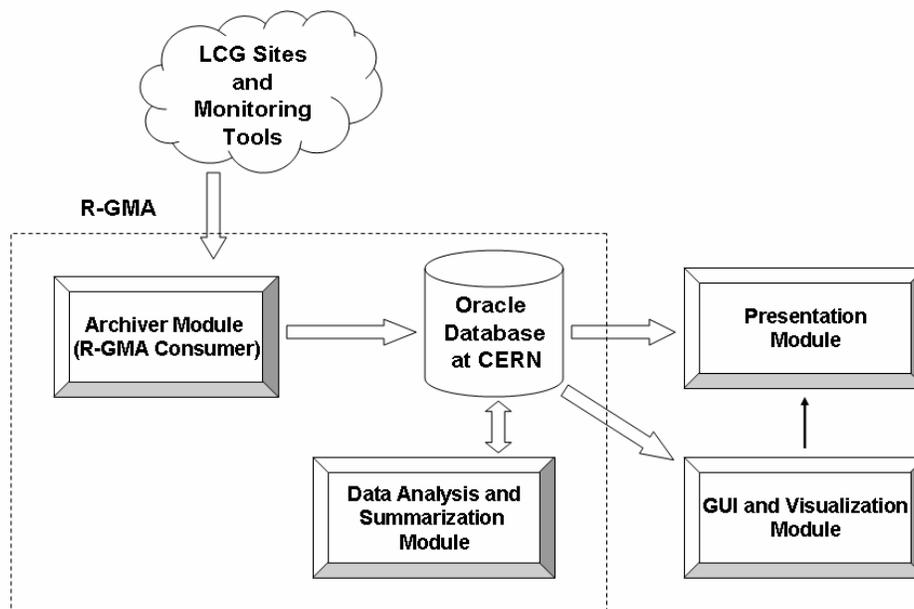
Figure 1: Block Schematic of Gridview Architecture
