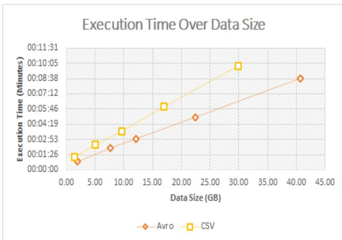
Figure 8b. Execution Time over Data Size. It represents the execution time over both Avro and CSV file data size.
