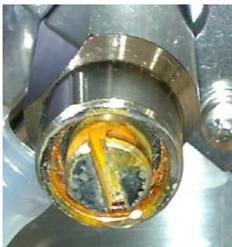
**Figure 4** The trace of corrosion on the drain valve after running the chiller with C6F14 and C6.
