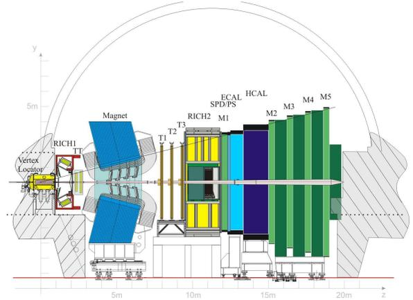
Fig. 1: Layout of the LHCb detector.
