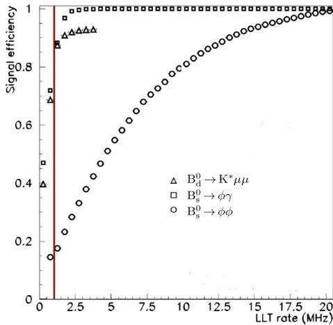
Fig. 6: LHCb upgrade trigger efficiency depending on the hardware trigger rate for  $B^0 \rightarrow K^{*0} \mu^+ \mu^-$ ,  $B_s^0 \rightarrow \phi \gamma$  and the purely hadronic  $B_s^0 \rightarrow \phi \phi$ .
