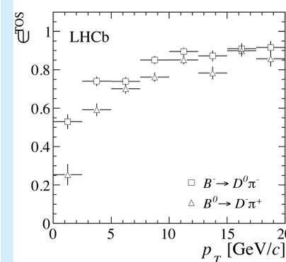
The efficiency of the Hlt2 topological  $n$ -body trigger for selected final states when at least one track from the decay satisfies the Hlt1 criteria. [V. V. Gligorov and M. Williams, (2013) JINST 8 P02013]
