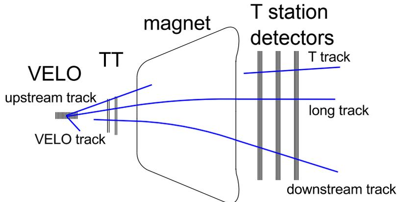
Figure 1: Illustration of the tracking system of LHCb, starting from the VELO around the collision point on the left, particles pass the TT, are deflected in the magnetic field of the dipole magnet and then detected in the T station detector (IT and OT). Different track types are reconstructed by different track finding algorithms. [1]
