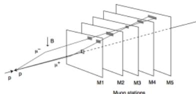
Fig. 4. Track finding by the Level-0 muon trigger. In the example shown,  $\mu^+$  and  $\mu^-$  cross the same pad in M3. Grey areas illustrate the field of interests used by the algorithm for station M1, M2, M4 and M5.
