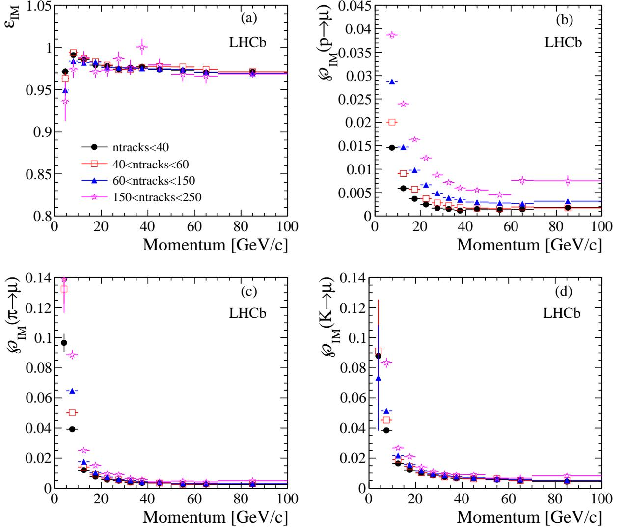
Figure 5: IsMuon efficiency  $\varepsilon_{IM}$  (a) and  $\wp_{IM}$  for protons (b), pions (c) and kaons (d) as a function of momentum for different ranges of the number of trajectories reconstructed in the event (ntracks).
