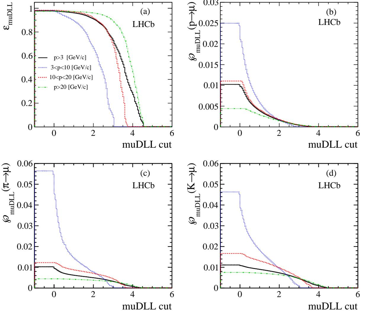
Figure 6: The efficiency  $\epsilon_{\text{muDLL}}$  as a function of muon DLL cut for muons (a) and misidentification probabilities for protons (b), pions (c) and kaons (d). The black solid line shows the average values integrated over  $p > 3 \text{ GeV}/c$ . The blue dotted line correspond to particles in the range  $3 < p < 10 \text{ GeV}/c$ . The red dashed lines show results for  $10 < p < 20 \text{ GeV}/c$  and the green dashed-dotted for  $p > 20 \text{ GeV}/c$ .
