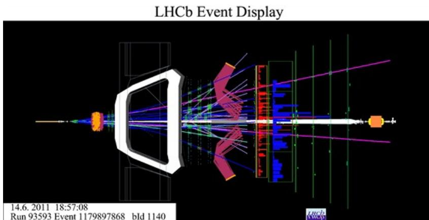
Figure 1: Schematic view of the LHCb experiment, displaying one event recorded in 2011, where 2 muons are identified (purple lines). This is one of the best  $B_s^0 \rightarrow \mu^+ \mu^-$  candidates selected from the 2011 data [3]. The muon stations are seen as the five green vertical lines, the second one placed just after the calorimeters, shown as the rectangles with red and blue bars representing the energy deposition along the direction transverse to the beam.
