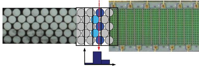
Fig. 1. Crosssections of fibre mat and multichannel SiPM. Determining the hit position by a weighted sum is indicated in the middle.
