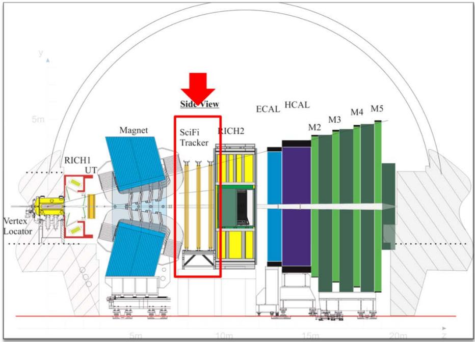
Figure 1: Overview: The SciFi tracker in the upgraded LHCb experiment.
