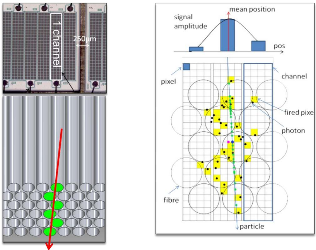
Figure 2: Principle of signal generation and detection.
