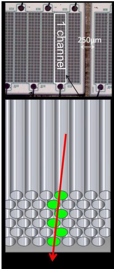
Figure 1: Principle of signal generation and detection in a close-packed 6-layer mat of scintillating fibres. The top part of the figure shows a close view of the SiPM array.
