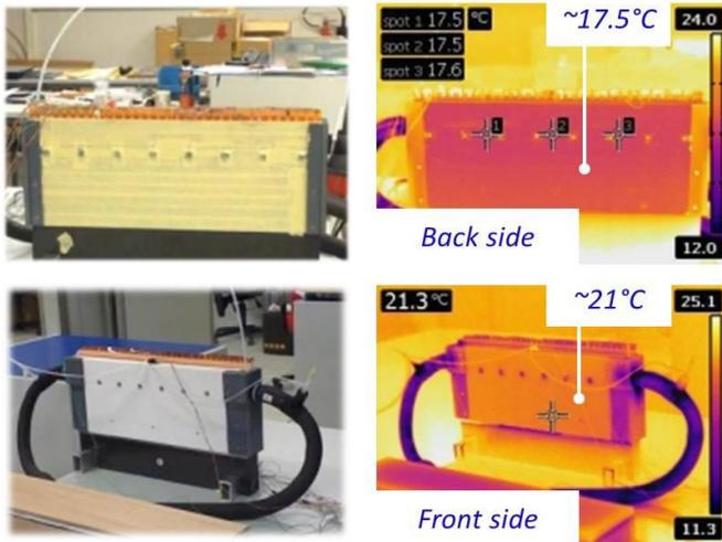
**Figure 7:** The IR images of the mock-up module running at  $-50^{\circ}\text{C}$ . Top: no extra insulation, the aluminium skin is covered with a paper tape; bottom: additional 10 mm layer of Rohacell insulation is added on top of the aluminium skin.
