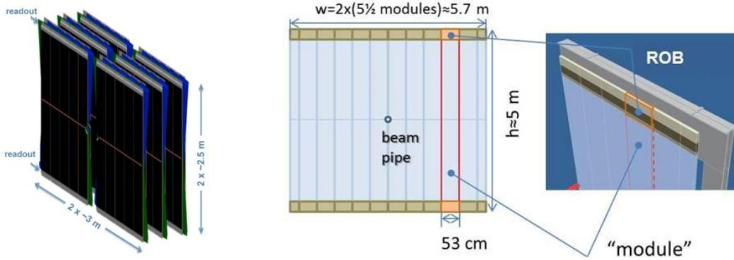
**Figure 1:** Left: schematic view of the SciFi tracker with 3 stations of X-U-V-X planes. Middle and right: a SciFi layer composed of “modules” each having the read-out boxes at the top and bottom ends. In X-planes the modules are vertical, while in stereo-angle U- and V-planes they are tilted at  $\pm 5^\circ$ .
