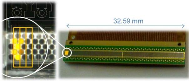
**Figure 2:** A custom-made 128-channel SiPM array with  $0.25 \times 1.32 \text{ mm}^2$  cells matching the fibre diameter and the thickness of the 5-layer ribbon. The SiPM signals are transferred to the front-end electronics via a flex PCB bonded to the SiPM package. There will be about 4600 such arrays in the whole SciFi tracker.
