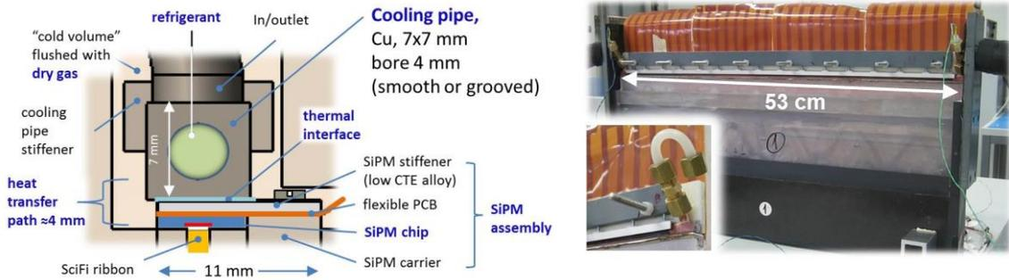
**Figure 4:** Left: schematic view of the SiPM-cooling interface region. Right: the mock-up module with the front cover removed, exposing the cold pipe, the pipe pressing mechanism and the dummy flex PCBs. The insert shows a detail of the cooling pipe edge with the outlet prepared for the serial connection with another module.
