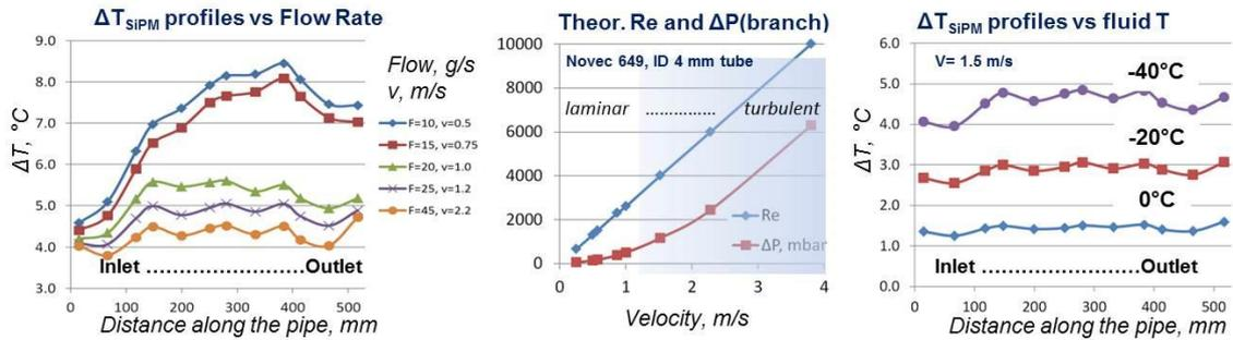
**Figure 6:** Temperature profiles for different fluid flow regimes. (a) Observed  $\Delta T_{SiPM}$  profiles along the pipe for the fluid at  $-45^\circ\text{C}$  and different flow rates. (b) Theoretical dependencies of the Reynolds number and the pressure drop over a cooling branch of 6 ROBs, on the fluid velocity. (c) Observed  $\Delta T_{SiPM}$  profiles for different fluid temperatures at  $v = 1.5$  m/s.
