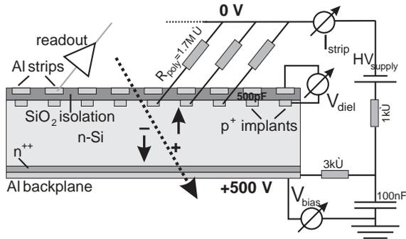
Fig. 1. Sensor schematics with electrical setup.
