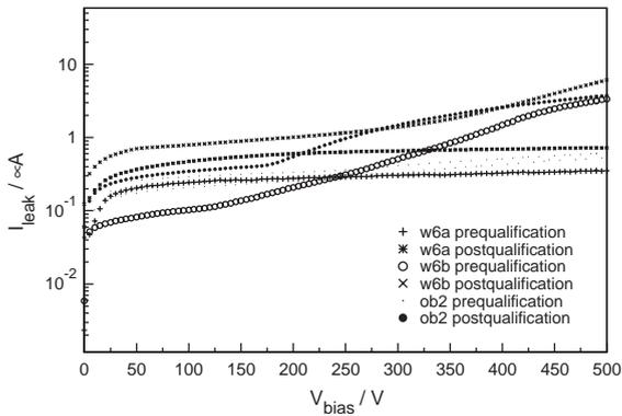
Fig. 4. Leakage current over bias voltage for three sensors before and after the test beam.
