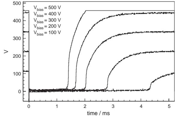
Fig. 2. Time behaviour of bias voltage.
