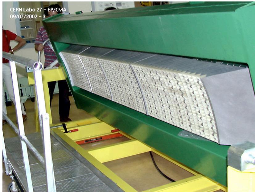
Figure 4.2: Photograph of supermodule, showing modules.
