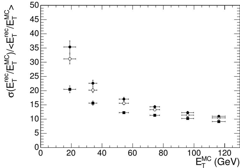
Figure 11.30: The jet  $E_T$  resolution as a function of generated jet  $E_T$  for reconstruction with calorimeter only (full circles), addition of out-of-cone tracks (open circles), and further charged track response corrections (full squares).
