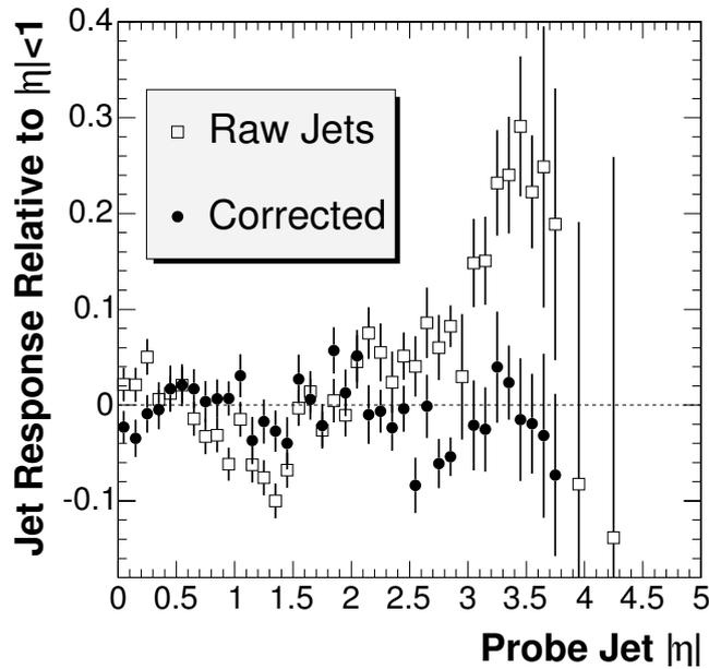
Figure 11.21: Jet response as a function of  $|\eta|$  for  $120 \text{ GeV}/c < \text{dijet } p_T < 250 \text{ GeV}/c$ . The graphs compares raw jets (open boxes) with corrected jets (solid circles). The indicated level of precision may be obtained on 1 hour of data taking.
