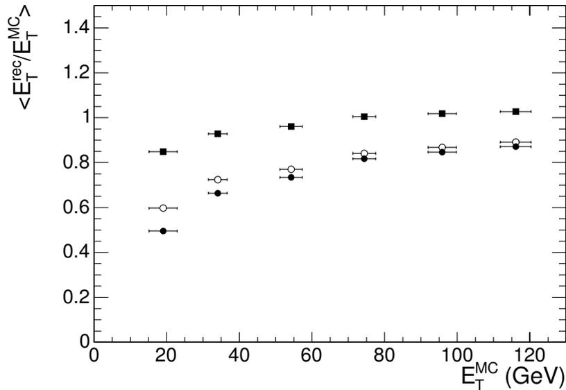
Figure 11.31: Ratio of reconstructed to generated jet  $E_T$  as a function of the generated jet  $E_T$  for reconstruction with calorimeter only (full circles), addition of out-of-cone tracks (open circles), and further charged track response corrections (full squares).
