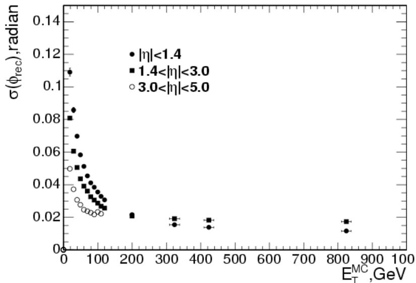
Figure 11.8: The jet  $\phi$  angular resolution as a function of the generated jet transverse energy for barrel jets ( $|\eta| < 1.4$ ), endcap jets ( $1.4 < |\eta| < 3.0$ ) and very forward jets ( $3.0 < |\eta| < 5.0$ ). The cuts  $E_T > 0.5$  GeV and  $E > 0.8$  GeV are used. The distance between generated and reconstructed jets is required to be  $\Delta R < 0.2$ .
