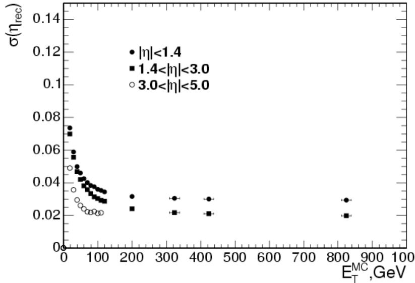
Figure 11.9: The jet  $\eta$  resolution as a function of the generated jet transverse energy for barrel jets ( $|\eta| < 1.4$ ), endcap jets ( $1.4 < |\eta| < 3.0$ ) and very forward jets ( $3.0 < |\eta| < 5.0$ ). The cuts  $E_T > 0.5$  GeV and  $E > 0.8$  GeV are used. The distance between generated and reconstructed jets is required to be  $\Delta R < 0.2$ .
