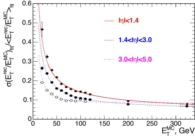
Figure 11.7: The jet transverse energy resolution as a function of the generated jet transverse energy for barrel jets ( $|\eta| < 1.4$ ), endcap jets ( $1.4 < |\eta| < 3.0$ ) and very forward jets ( $3.0 < |\eta| < 5.0$ ). The jets are reconstructed with the iterative cone  $R = 0.5$  algorithm. The cuts  $E_T > 0.5$  GeV and  $E > 0.8$  GeV are used. The distance between generated and reconstructed jets is required to be  $\Delta R < 0.2$ . The Monte Carlo jet calibration has been applied.
