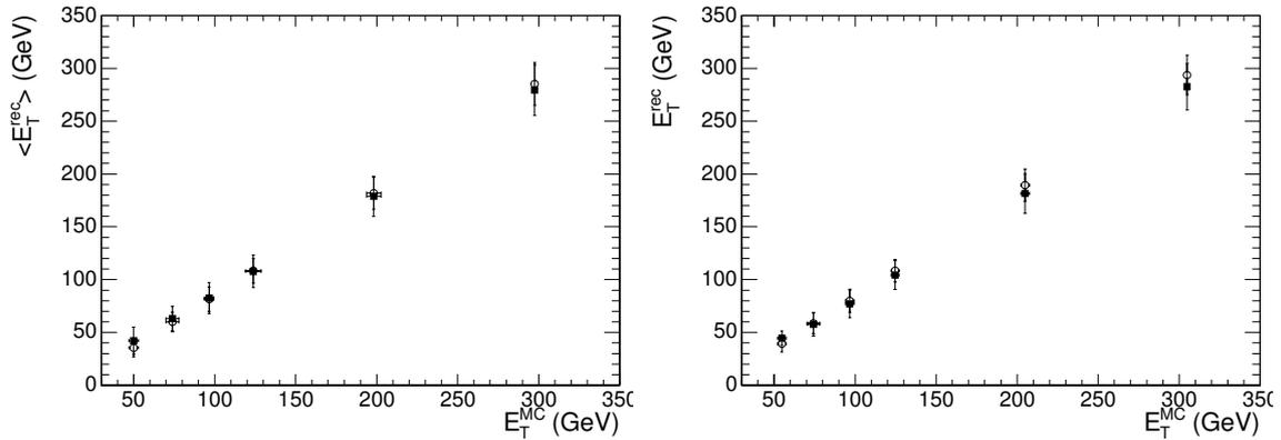
Figure 11.33: The correlation between the average reconstructed and the generated jet transverse energies in Pb-Pb (full squares) and  $pp$  (open circles) events in the barrel (left) and endcap (right). The error bars are the dispersion of jet energy distribution.
