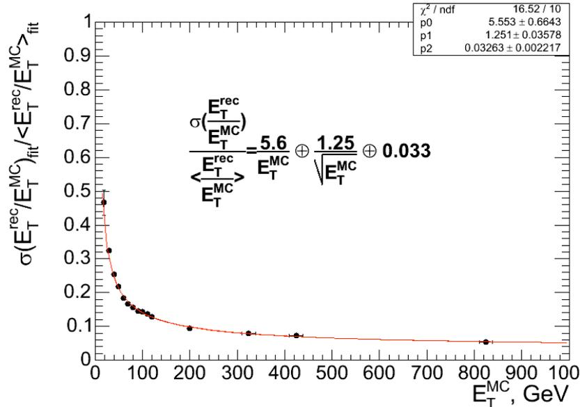
Figure 11.6: The jet transverse energy resolution as a function of the generated jet transverse energy for barrel jets ( $|\eta| < 1.4$ ). The cuts  $E_T > 0.5$  GeV and  $E > 0.8$  GeV are used. The distance between generated and reconstructed jets is  $\Delta R < 0.2$ . The Monte Carlo jet calibration has been applied.
