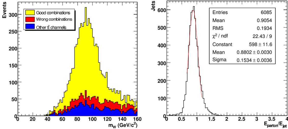
Figure 11.29: Distribution of the  $W$  boson mass including combinatorial and process backgrounds, together with the distribution of  $E_{\text{parton}}/E_{\text{jet}}$  obtained from simulation truth. The background samples are rescaled to the integrated luminosity of the signal sample.
