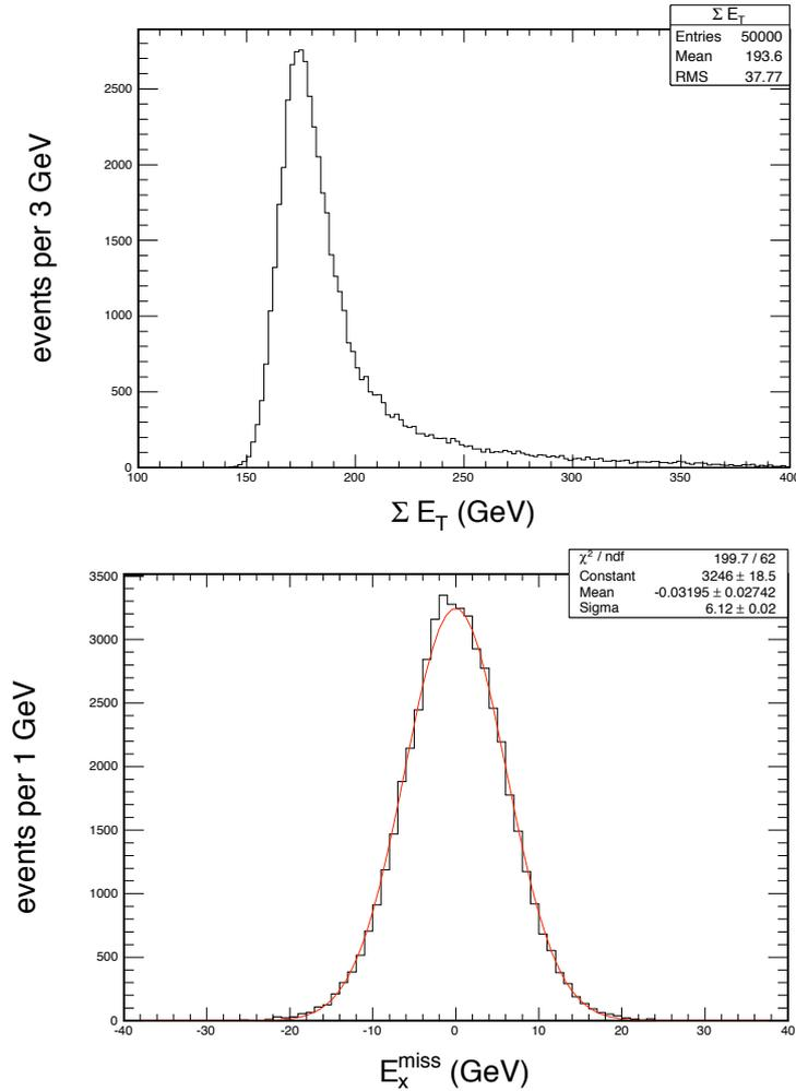
Figure 11.10: Top) Distribution of  $\Sigma E_T$  and Bottom)  $E_x^{\text{miss}}$  for minimum bias events with no pile-up. The resolution is 6.1 GeV in agreement with expectations based on a stochastic term of  $0.65\sqrt{\Sigma E_T}$  GeV<sup>1/2</sup> and a noise contribution of 3.8 GeV.
