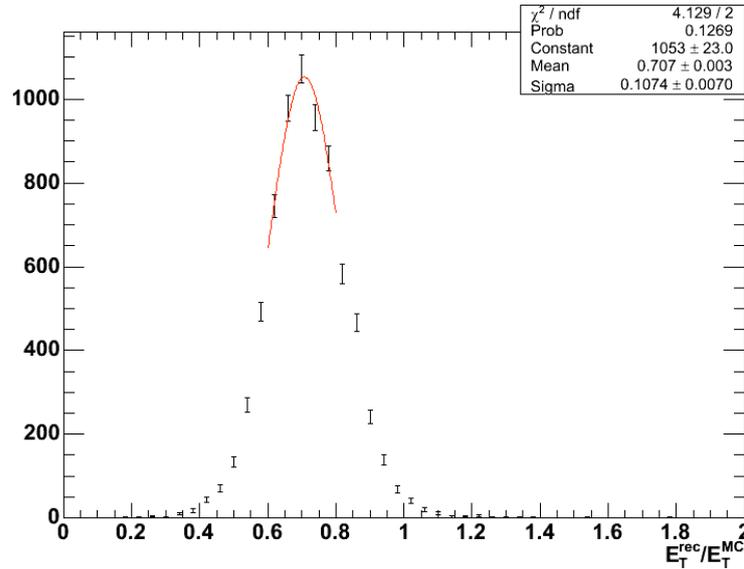
Figure 11.5: Distribution of reconstructed jet transverse energy ( $E_T^{\text{rec}} = p_T^{\text{rec}} c$ ) divided by particle-level generated jet transverse energy ( $E_T^{\text{MC}} = p_T^{\text{MC}} c$ ) for generated jets in the range  $105 \text{ GeV} < E_T^{\text{MC}} < 115 \text{ GeV}$ . The jets are reconstructed with the iterative cone  $R = 0.5$  algorithm.
