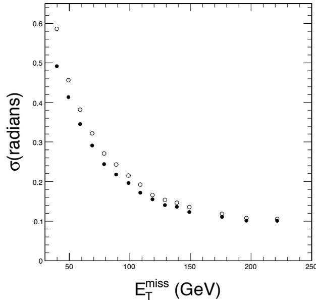
Figure 11.20: Error in the direction of the vector  $\mathbf{E}_T^{\text{miss}}$  as a function of reconstructed  $E_T^{\text{miss}}$  in inclusive  $t\bar{t}$  events before (open circles) and after corrections (filled circles).
