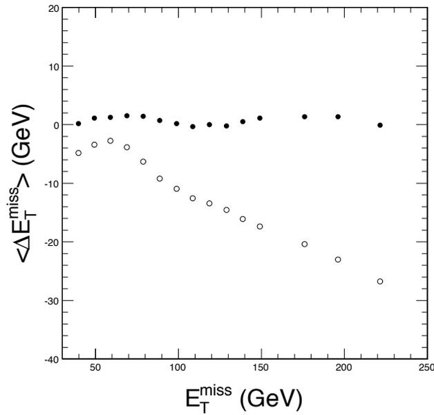
Figure 11.19: Error in the reconstructed missing transverse energy scale before (open circles) and after jet corrections (filled circles) for inclusive  $t\bar{t}$  events vs. reconstructed  $E_T^{\text{miss}}$ .
