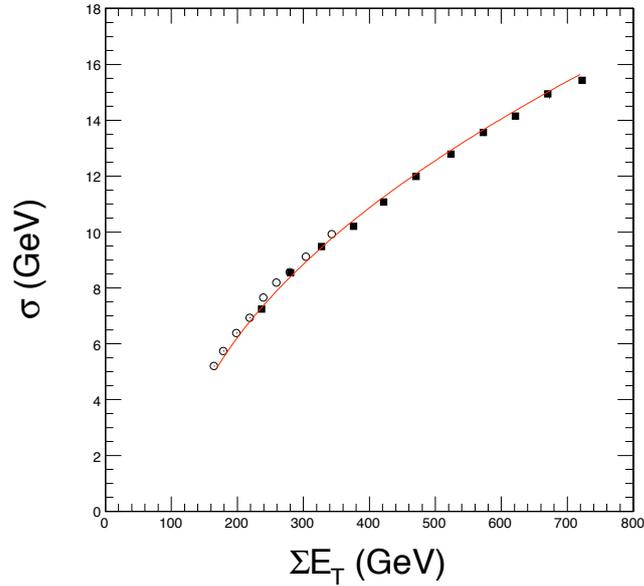
Figure 11.12: Missing transverse energy resolution vs.  $\Sigma E_T$  for QCD soft events,  $0 < \hat{p}_T < 15 \text{ GeV}/c$ , (squares) and minimum bias events (open circles). Low-luminosity pile-up is included in both cases.
