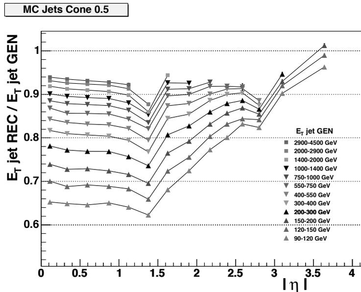
Figure 11.4: The ratio of the reconstructed jet transverse energy  $E_T^{\text{rec}}$  to the generated transverse energy  $E_T^{\text{MC}}$  as a function of generated jet  $\eta$  for jets with different  $E_T^{\text{MC}}$  reconstructed by the iterative cone  $R = 0.5$  algorithm before Monte Carlo corrections.
