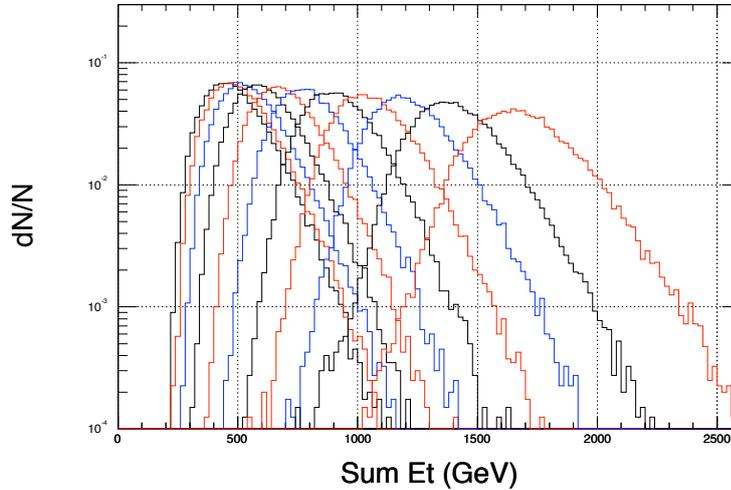
Figure 11.13: Distribution of  $\Sigma E_T$  observed in the detector for QCD events corresponding to  $\hat{p}_T$  ranges (from left to right) of 20-30, 30-50, 50-80, 80-120, 120-170, 170-230, 230-300, 300-380, 380-470, 470-600 and 600-800  $\text{GeV}/c$ .
