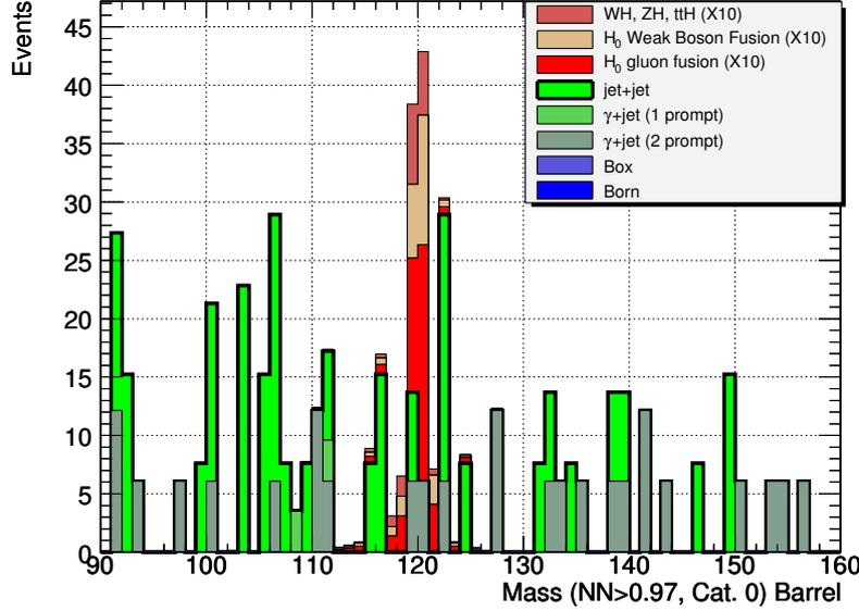
Figure 2.8: The diphoton mass distribution for each source for barrel events with kinematic neural net output greater than 0.97 and  $R_9 > 0.948$ . Events are normalised to an integrated luminosity of  $7.7 \text{ fb}^{-1}$  and the Higgs signal ( $M_H=120 \text{ GeV}/c^2$ ) is scaled by a factor 10.
