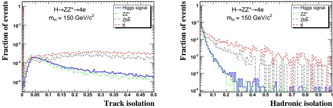
Figure 2.14: Electron isolation observables for the signal at  $m_H = 150 \text{ GeV}/c^2$  and the SM backgrounds; a) track isolation,  $\sum_{\text{cone}} p_T^{\text{tracks}} / p_T^e$ ; b) hadronic isolation,  $\sum_{\text{cone}} E_T^{\text{HCAL}} / p_T^e$ , for the second least isolated electrons.
