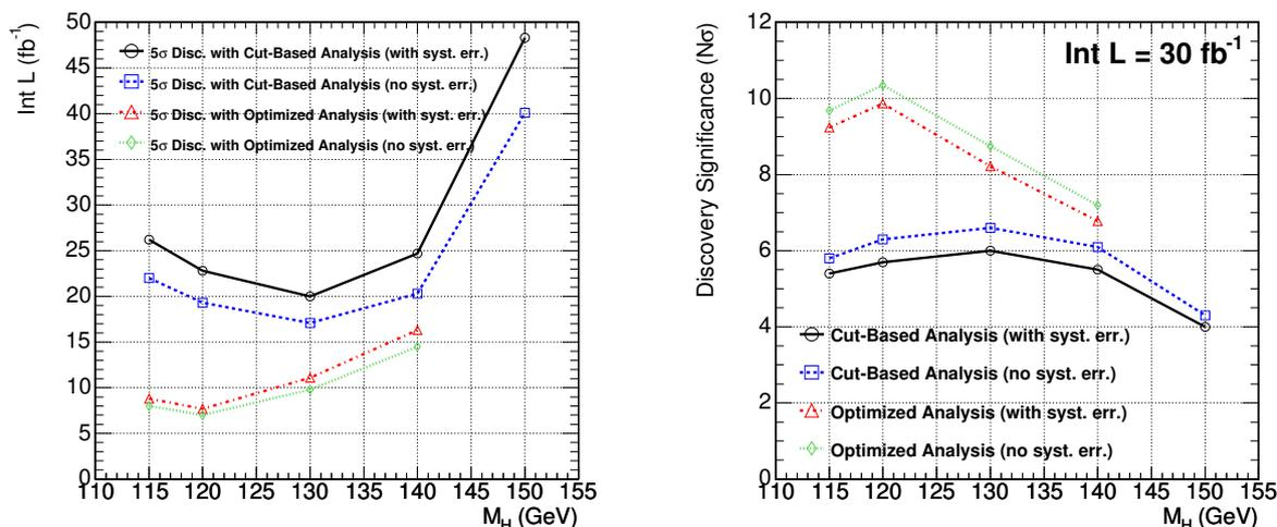
Figure 2.10: Integrated luminosity needed for a  $5\sigma$  discovery (left) and discovery sensitivity with an integrated luminosity of  $30 \text{ fb}^{-1}$  (right) with the optimised analysis. The results from the cut-based analysis in 12 categories are also shown for comparison.
