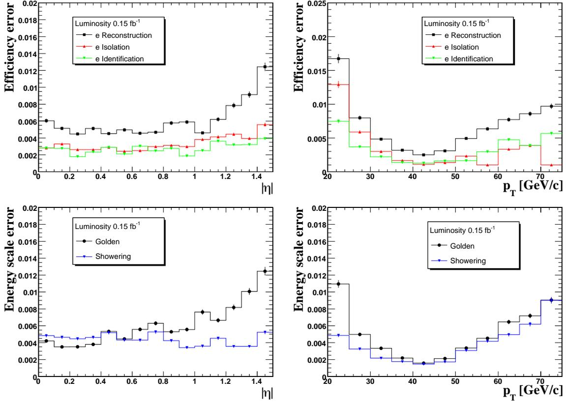
Figure 2.17: Control of experimental uncertainties using SM data; uncertainties on measurements of electron reconstruction, isolation and identification as a function of (a)  $\eta$  and (b)  $p_T$ ; uncertainties on measuring the energy scale for golden and showering electrons as a function of (c)  $\eta$  and (d)  $p_T$ .
