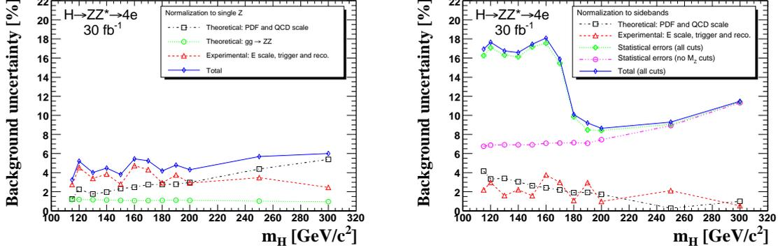
Figure 2.18: Theoretical and experimental uncertainty estimations for both methods for evaluation of background from data: (a) normalisation to the single  $Z \rightarrow 2e$  measurements and (b) normalisation to the sidebands. Expected statistical errors for sidebands are also shown, for integrated luminosity of  $30 \text{ fb}^{-1}$ .
