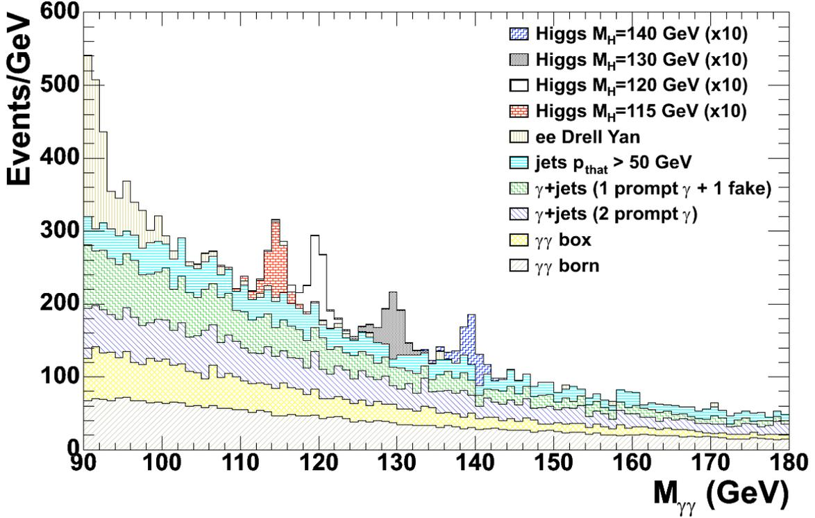
Figure 2.2: Diphoton invariant mass spectrum after the selection for the cut-based analysis. Events are normalised to an integrated luminosity of  $1 \text{ fb}^{-1}$  and the Higgs signal, shown for different masses, is scaled by a factor 10.
