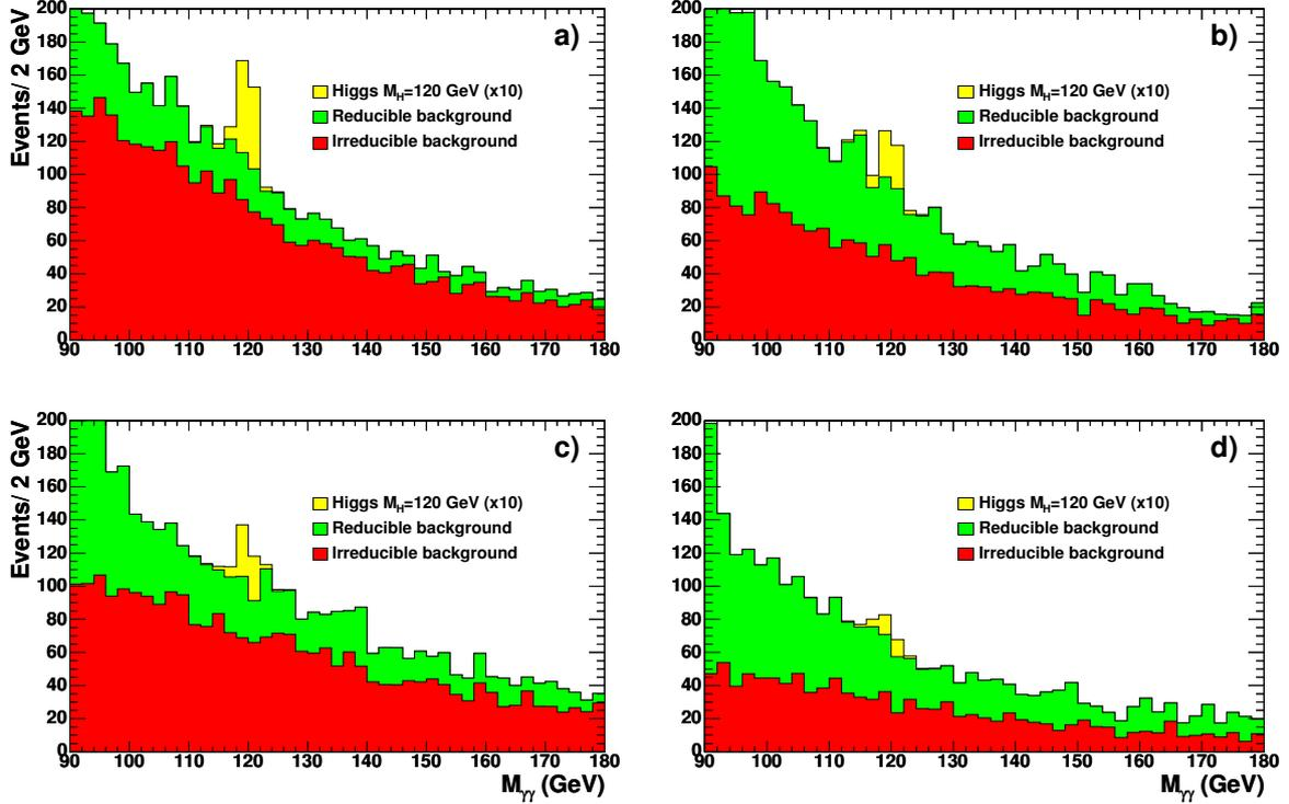
Figure 2.3: Invariant mass spectrum after the selection relative to the cut-based analysis with four categories defined in the text: barrel with large  $R_9$  (a), barrel with small  $R_9$  (b), endcaps with large  $R_9$  (c) and endcaps with small  $R_9$  (d), Events are normalised to an integrated luminosity of  $1 \text{ fb}^{-1}$  and the Higgs signal, shown for different masses, is scaled by a factor 10.
