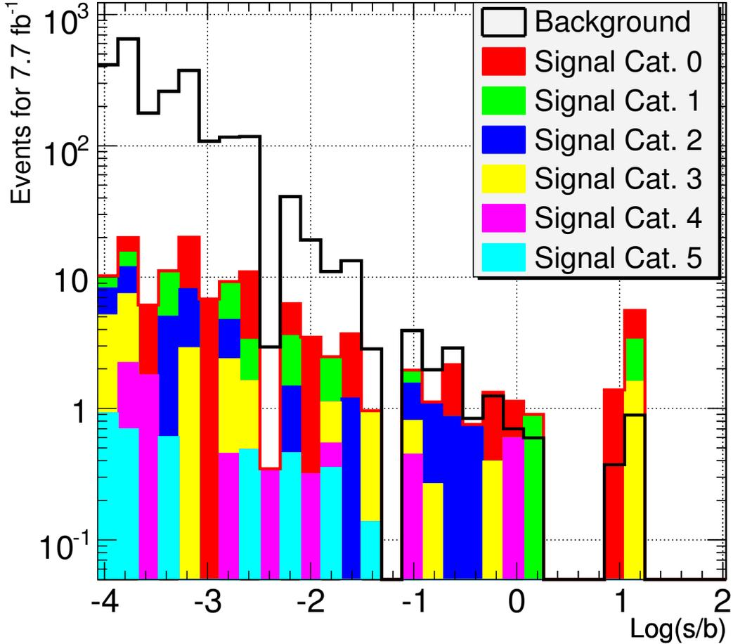
Figure 2.9: The final distribution of binned signal ( $M_H=120\text{ GeV}/c^2$ ) and background in  $\log(s/b)$  for an integrated luminosity of  $7.7\text{ fb}^{-1}$ . Here the Higgs signal is normalised to the integrated luminosity and the statistics benefits of the smoothing of the background. Signal and background events are added independently.
