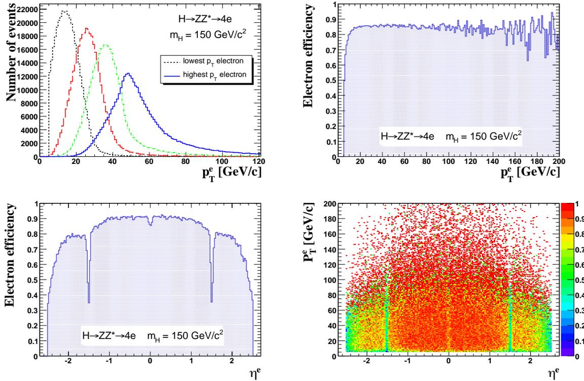
Figure 2.11: Electrons in SM Higgs boson  $4e$  decay channel for  $m_H = 150 \text{ GeV}/c^2$ ; a) transverse momentum of each of the four final state electrons; b) efficiency at pre-selection as a function of  $p_T^e$ ; c) efficiency at pre-selection as a function of  $\eta_e$ ; d) efficiency in the  $p_T^e$  versus  $\eta_e$  plane.
