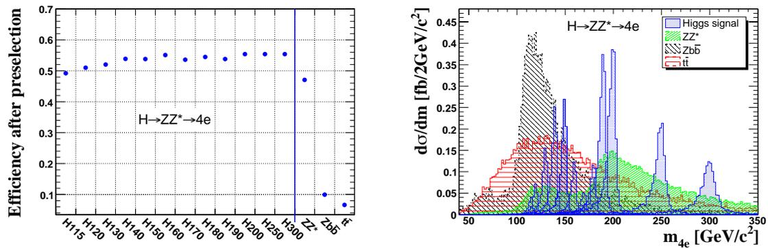
Figure 2.12: Higgs boson signal and dominant background sources after pre-selection step; a) overall pre-selection efficiency for  $m_H$  in the range from 115 to 300 GeV/c<sup>2</sup> and the background from  $ZZ^{(*)}$  continuum, from  $Zb\bar{b}$  and  $t\bar{t}$ ; b) separate signal and background contributions to the spectrum of reconstructed invariant mass  $m_{4e}$ .
