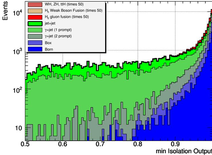
Figure 2.4: Distribution of the minimum value of the  $NN_{\text{isol}}$  variables of the two photon candidates. Events are normalised to an integrated luminosity of  $7.7 \text{ fb}^{-1}$  and the signal ( $M_H=120 \text{ GeV}/c^2$ ) is scaled by a factor 50.
