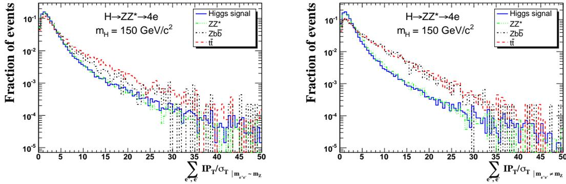
Figure 2.13: Sum of the transverse impact parameter significance ( $IP_T/\sigma_T$ ) of  $e^+e^-$  pairs for a Higgs boson at  $m_H = 150 \text{ GeV}/c^2$ , for the  $ZZ^{(*)}$  continuum, and for  $Zb\bar{b}$  and  $t\bar{t}$ ; a)  $\sum IP_T/\sigma_T$  from the electrons of the  $e^+e^-$  pair with a reconstructed mass  $m_{ee}$  best matching the Z boson mass; b)  $\sum IP_T/\sigma_T$  from the second  $e^+e^-$  pair.
