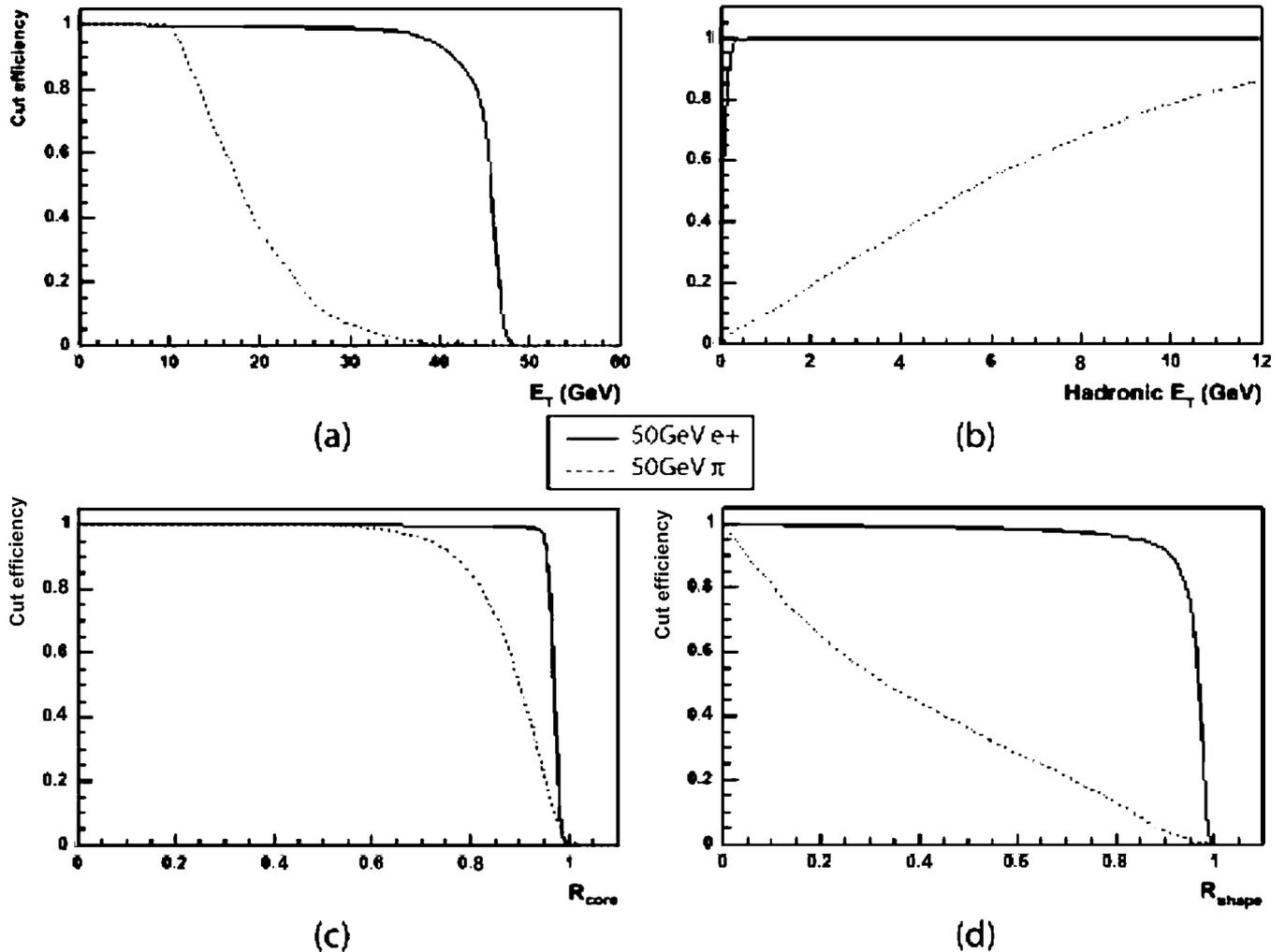
Fig. 4. Study  $e/\pi$  separation with 2004 CTB data using the LVL2 calorimeter and tracking algorithms. (a) Cut efficiency at the first step of T2Calo algorithm. (b) Cut efficiency at the second step of T2Calo. (c) Cut efficiency at the third step of T2Calo. (d) Cut efficiency at the last step of T2Calo.
