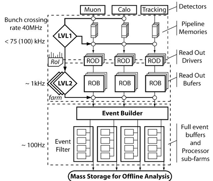
Fig. 1. Block diagram of the ATLAS Trigger/DAQ system.
