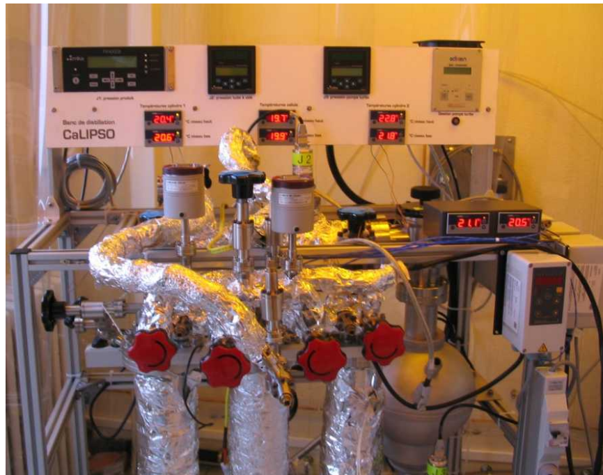
Batch (r.) and column (u.) ultrapurification stations
