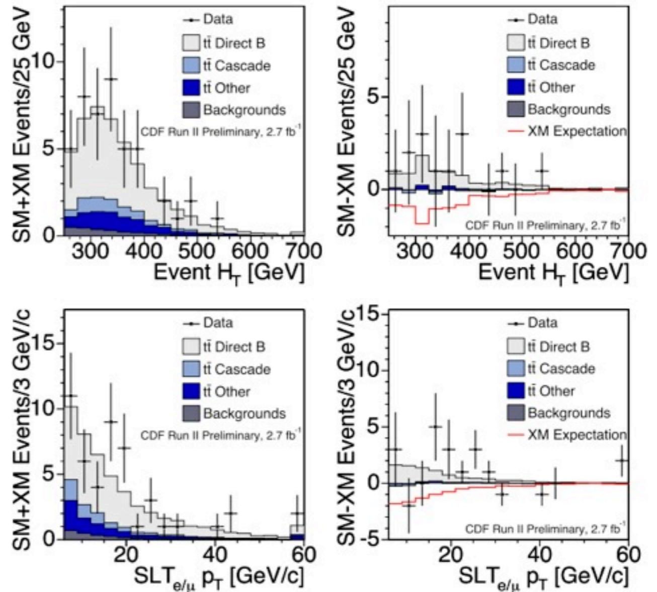
FIG. 1: Distribution of the SM+XM (left) and SM-XM tags (right) as a function of the event  $H_T$  (top) and SLT track  $p_T$  (bottom). The total  $t\bar{t}$  contribution is normalized to the data. Contributions from direct semileptonic decay of  $b$ -jets, semileptonic cascade decays and other sources of SLT tags are shown separately, along with the expected SM background. The expectation for a hypothetical XM top is shown in red.
