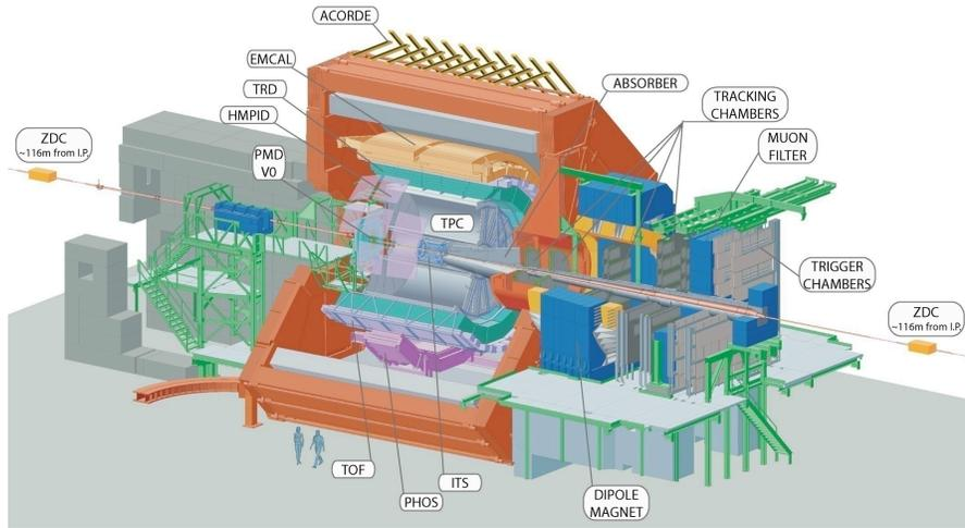
**Figure 1.** General layout of the ALICE detector.
