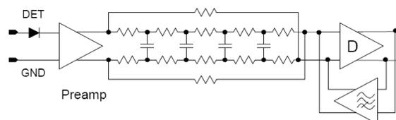
Fig. 5: The constant fraction discriminator. The two cross-connected resistors generate the signal fraction while the cascaded low-pass filters generate the delay.
