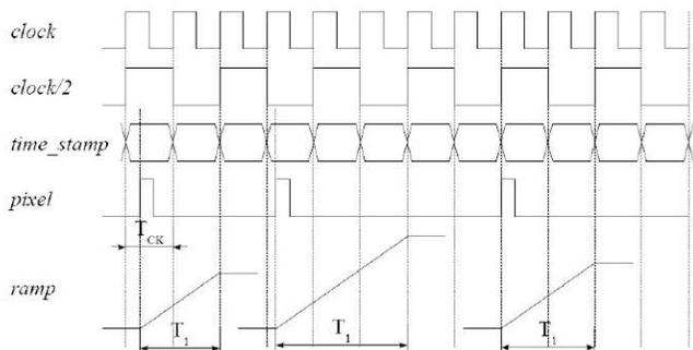
Fig. 1. Relevant timing waveforms used in the ASIC.
