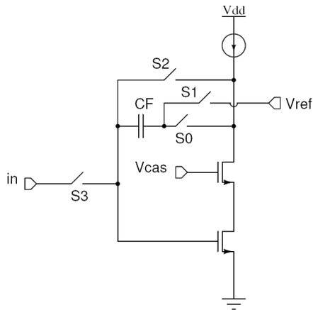
Fig. 9: The Time to Amplitude Converter.
