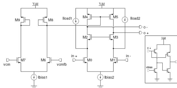
Fig. 4: Transistor level implementation of the core amplifier used in the front-end. The class AB output stage is shown in the inset.
