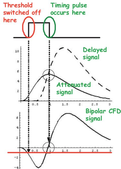
Fig. 7: Relevant waveforms for the circuit of Fig. 6
