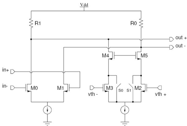
Fig. 6: Schematic of the zero crossing detector used in the CFD.
