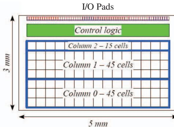
Fig. 2. Floorplan and size of the designed prototype.
