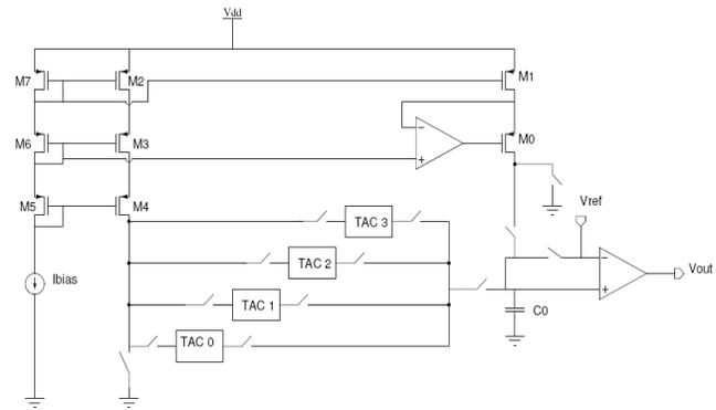
Fig. 10: Simplified schematic of the full TDC.
