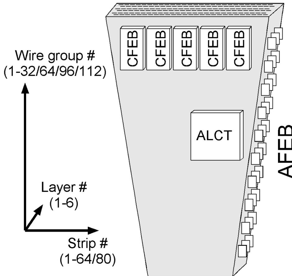
Figure 3. A view of a (non-ME1/1) CSC chamber with electronics on top and the corresponding definition of local CSC coordinates. (\*\*\*) Note that the number of wire groups is 1-32/48/64/96/112. Awaiting figure update using Canvas software)
