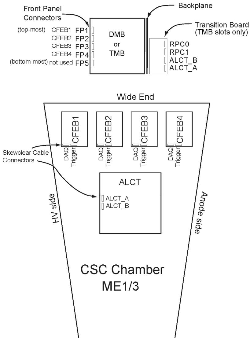
Figure 18. Cable connections for ME1/3 chambers.
