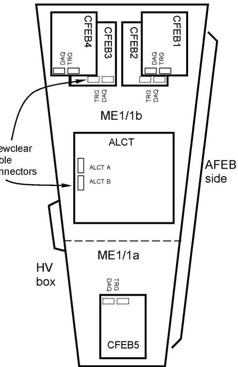
3. Figure 19 shows connections for ME1/1 (a and b sub-chambers).
