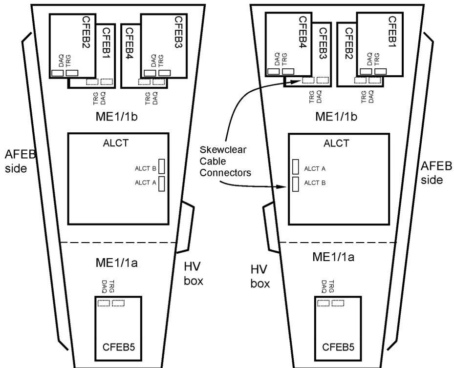
Figure 19. Cable connections for ME1/1 chambers (ME1/1a and ME1/1b sub-chambers).
