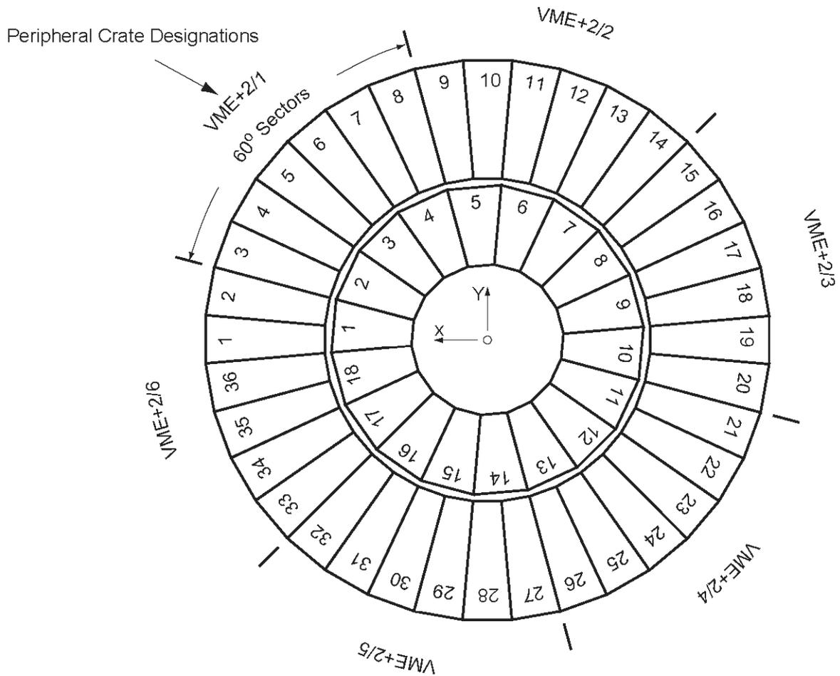
**Figure 10.** An  $r$ - $\phi$  cross-section of the ME2, ME3, and ME4 endcap muon stations viewed from  $z$ =negative infinity, showing the positions of chambers, trigger sectors, and correspondence to peripheral crate names, denoted as VME<station>/<phi index>. On the + $z$  side, this is the same view as *from* the IP, while on the - $z$  side, this is a view looking *towards* the IP.
