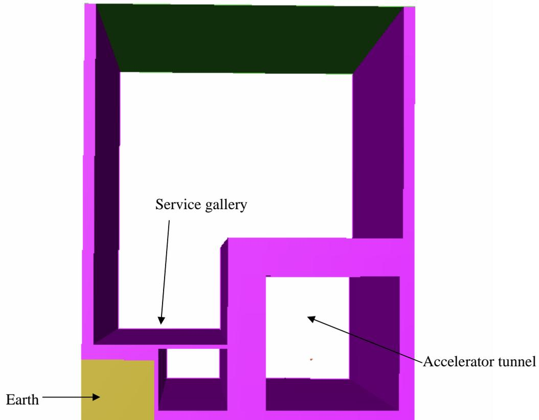
**Figure 2:** The high-energy section of the Linac 4 tunnel in building 363 as coded in FLUKA and visualised via the SimpleGeo geometry package [9]. The view is looking downstream of the tunnel, towards the transfer line.
