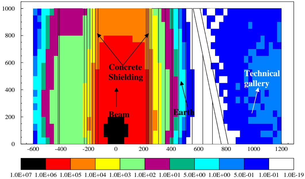
**Figure 7:** Beam loss in a  $5 \times 5 \times 5 \text{ cm}^3$  copper target, 10 W, 140 MeV. Top cross sectional view of the Linac 4 tunnel and of building 351.  $H^*(10)$  in  $\mu\text{Sv/h}$  on the ground floor.
