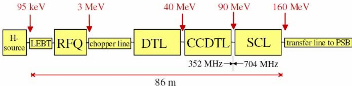
**Figure 1:** Schematic view of Linac 4.
