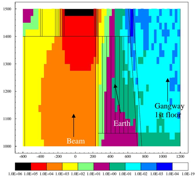
**Figure 10:** Beam loss in a  $5 \times 5 \times 5 \text{ cm}^3$  copper target, 10 W, 160 MeV. Top cross sectional view of the Linac 4 tunnel and of building 351.  $H^*(10)$  in  $\mu\text{Sv/h}$  at 530 cm above the hall floor where the gangway is located.
