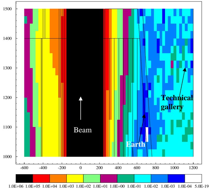
**Figure 9:** Beam loss in a  $5 \times 5 \times 5 \text{ cm}^3$  copper target, 10 W, 160 MeV. Top cross sectional view of the Linac 4 tunnel and of building 351.  $H^*(10)$  in  $\mu\text{Sv/h}$  on the ground floor where the Linac 3 technical gallery is located.
