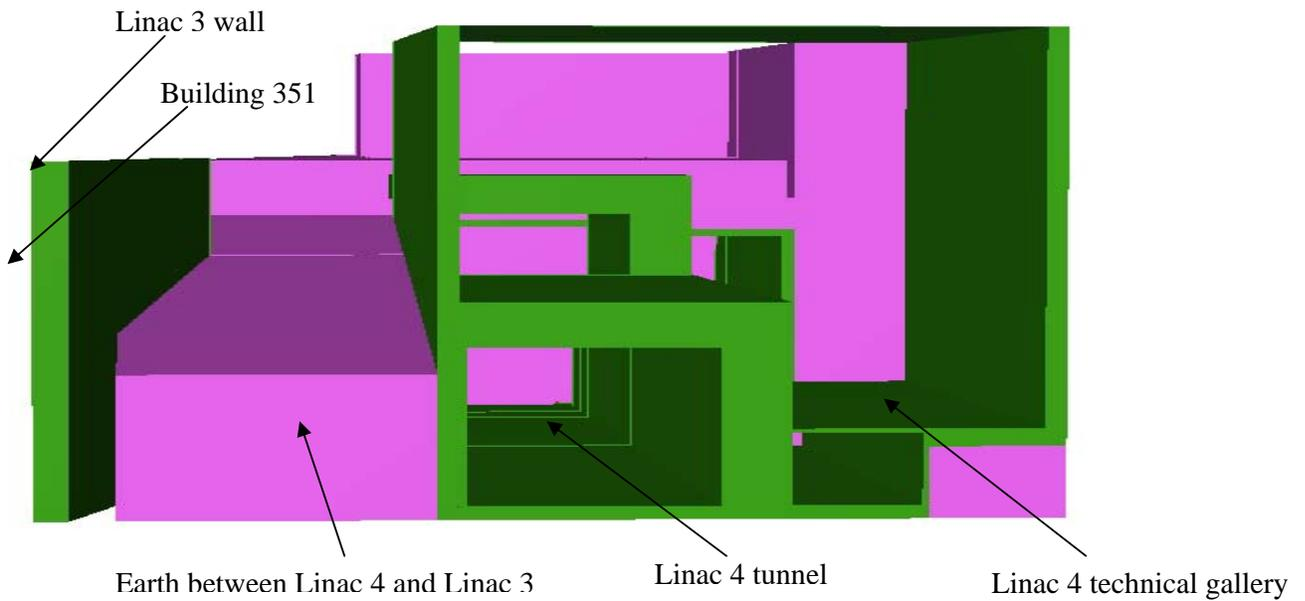
**Figure 5:** SimpleGeo [9] front view of the Linac 4 building and the wall of building 351. The view is looking upstream of the tunnel, towards the high-energy end of the linac.
