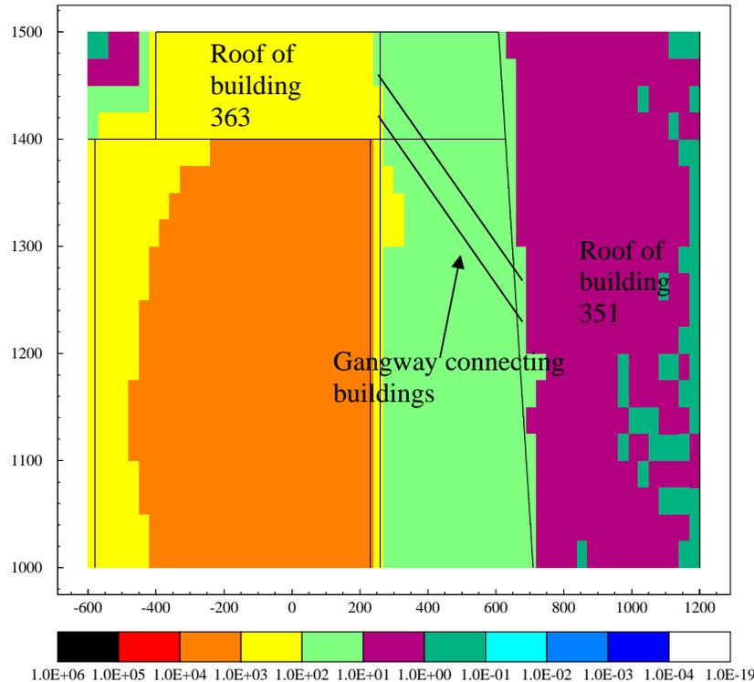
**Figure 11:** Beam loss in a  $5 \times 5 \times 5 \text{ cm}^3$  copper target, 10 W, 160 MeV. Top cross sectional view of the Linac 4 tunnel and of building 351.  $H^*(10)$  in  $\mu\text{Sv/h}$  at 760 cm above the hall floor where the gangway connecting the two buildings is located.
