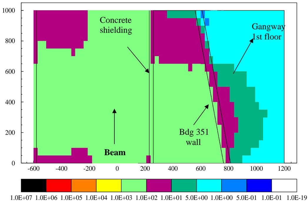
**Figure 8:** Beam loss in a  $5 \times 5 \times 5 \text{ cm}^3$  copper target, 10 W, 140 MeV. Top cross sectional view of the Linac 4 tunnel and of building 351.  $H^*(10)$  in  $\mu\text{Sv/h}$  at 530 cm above the hall floor where the gangway is located.
