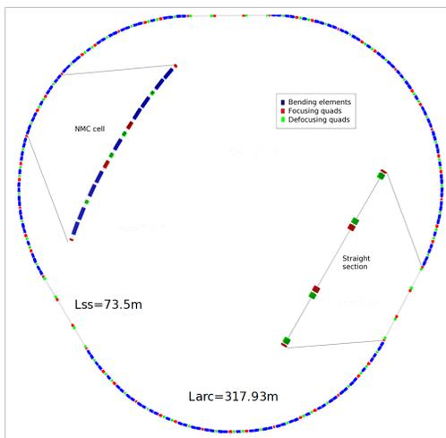
Figure 1: Schematic layout of the HP-PS ring.
