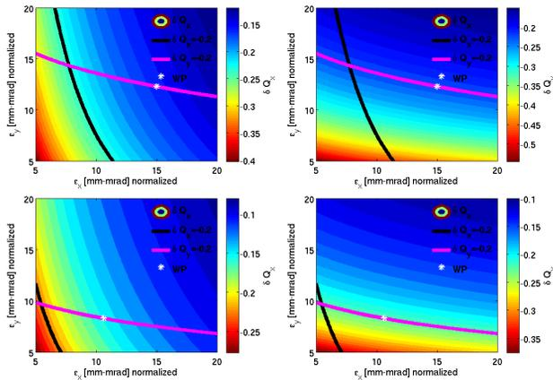
Figure 3: Horizontal versus vertical normalised emittance colour-coded with the horizontal (left) and vertical (right) space charge tune-shift for a Gaussian bunch, for the HP-PS option of 50 (top) and 75 GeV (bottom). The black and purple curves correspond to the horizontal and vertical space charge limit of -0.2.
