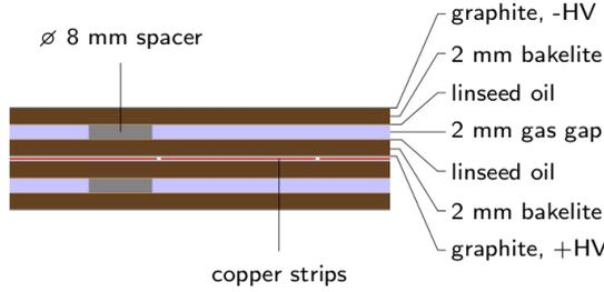
Fig. 2. The structure of the RPC detector. The double gas-gaps and the sandwich readout strip scheme will provide high efficiency.
