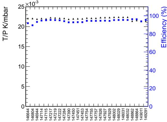
Fig. 9. (color online) Average RPC efficiency with respect to the run numbers. The efficiency fluctuation is correlated to the temperature and pressure variation.
