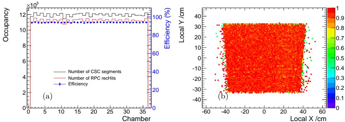
Fig. 5. (color online) RPC efficiency distribution from MC simulation, the CSC segment cone criteria was applied. The analysis of RE+1/3/b MC data is shown here as an example: (a) RPC efficiency and the occupancies of both RPC and CSC versus chamber number of all 36 chambers in the ring, (b) the merged 2D efficiency distributions on RPC surface.
