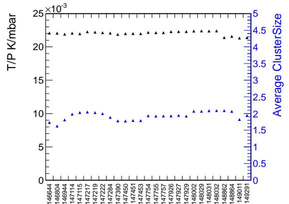
Fig. 12. (color online) The average cluster size with respect to run number or environmental parameters, showing the correlation with the pressure and temperature fluctuation. The error corresponds to the RMS of the cluster size.
