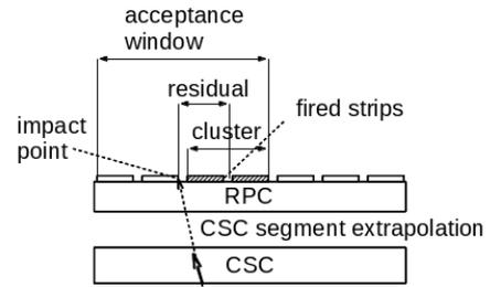
Fig. 3. CSC track segment extrapolation: the impact position is evaluated by extrapolate a single CSC track segment straightly to the corresponding RPC detector surface. Residual between the fire position and the impact position is measured, and an acceptance windows is applied to determine the efficiency.
