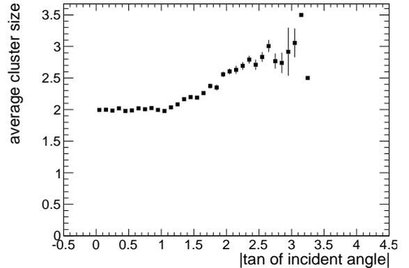
Fig. 11. Correlation between the average cluster size and the incident angle on RE+1/3/b. The error corresponds to the RMS of the cluster size within each bin.
