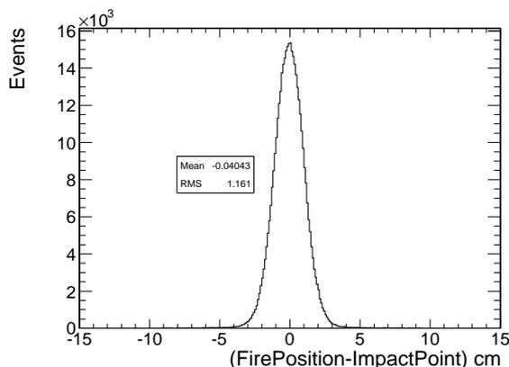
Fig. 13. Residual distributions: the distance between the RPC fired strip and the impact po-
