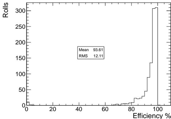
Fig. 7. Efficiency distribute on all RPC rolls from 2010 data at  $HV = 9500V$ .
