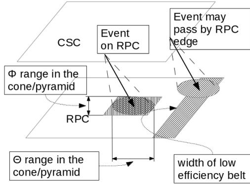
Fig. 4. The definition of CSC track segment cone in extrapolation used to estimate measurement bias. The cone projection indicates if the actual trajectory could possibly pass by the edge of RPC surface.
