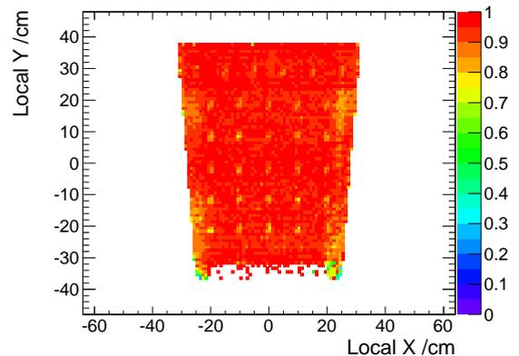
Fig. 8. (color online) Merged 2D efficiency distributions over the RE+1/2/a surfaces, for all 2010 data at  $HV = 9500V$ . The regularly distributed low efficiency spots correspond to the spacers inside the gas gap structure.
