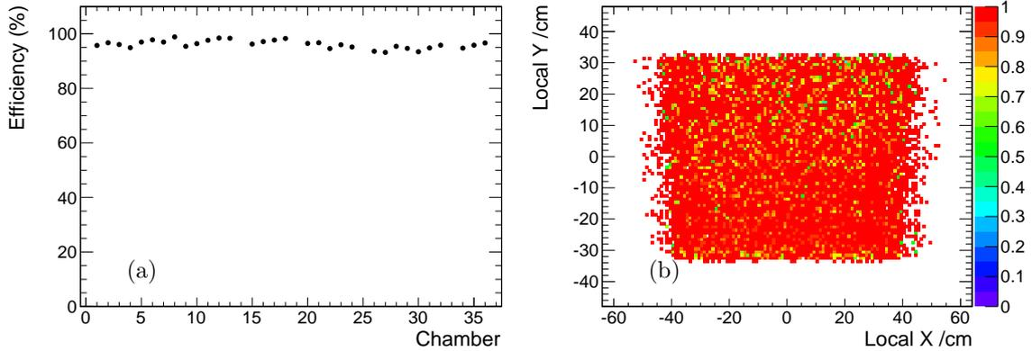
Fig. 6. (color online) RPC efficiency distribution from collision data (run 147755, luminosity is  $0.5153pb^{-1}$ , HV was set at 9500V). The RE+1/R3 roll b data is shown here as an example: (a) efficiency versus chamber number of all 36 chambers in the ring, the masked chambers are removed from calculation. Low efficiency chambers mostly worked in single gap mode; (b) merged 2D efficiency distributions on RPC surface.
